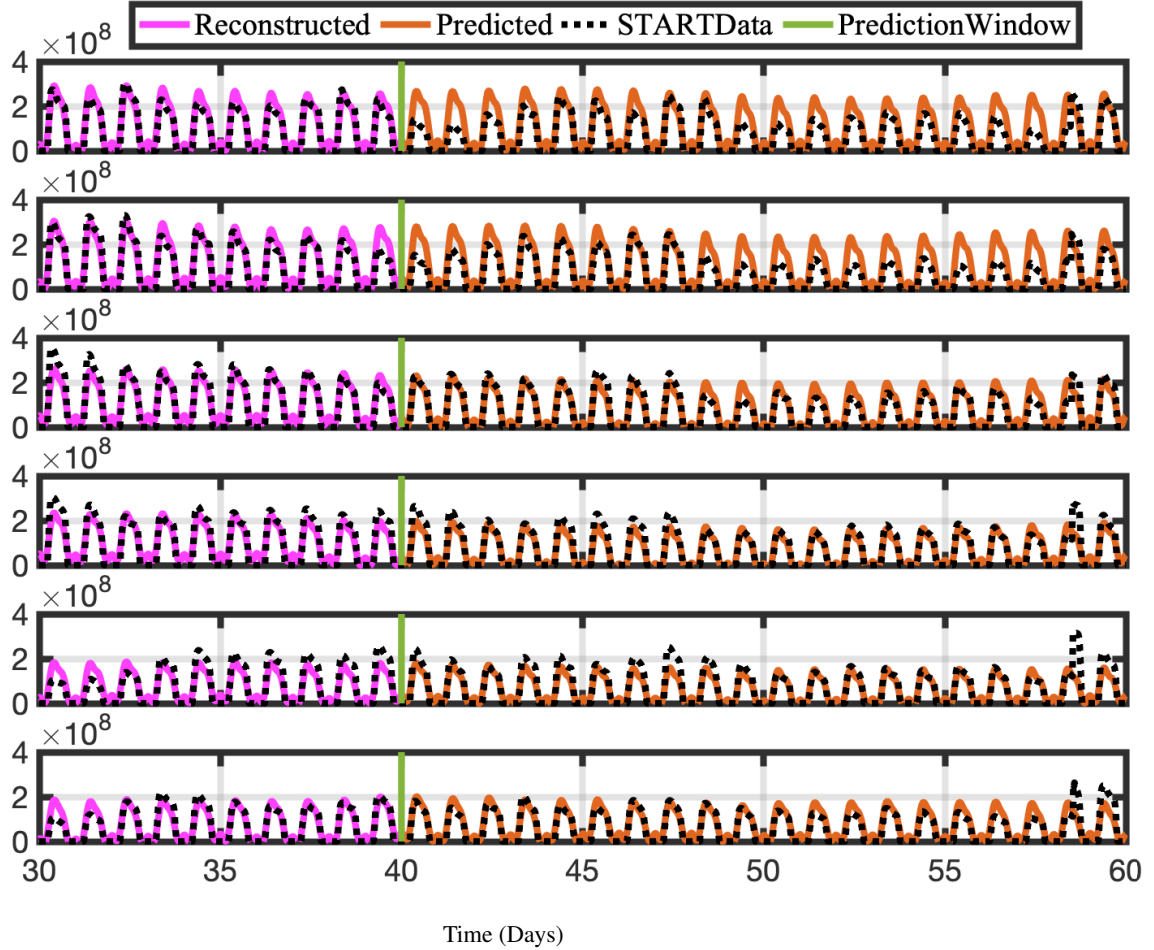
Figure 12. Time series of reconstructed and predicted results with \text{NO}_{\text{CONC}} data at Lat 30^\circ and 6 longitudes -180^\circ:5^\circ:-155^\circ . Both the reconstructed data, shown here for 10 days; and the forecasted time series, shown here for the 20 day testing period, reproduce the actual data for \text{NO}_{\text{CONC}} well.
