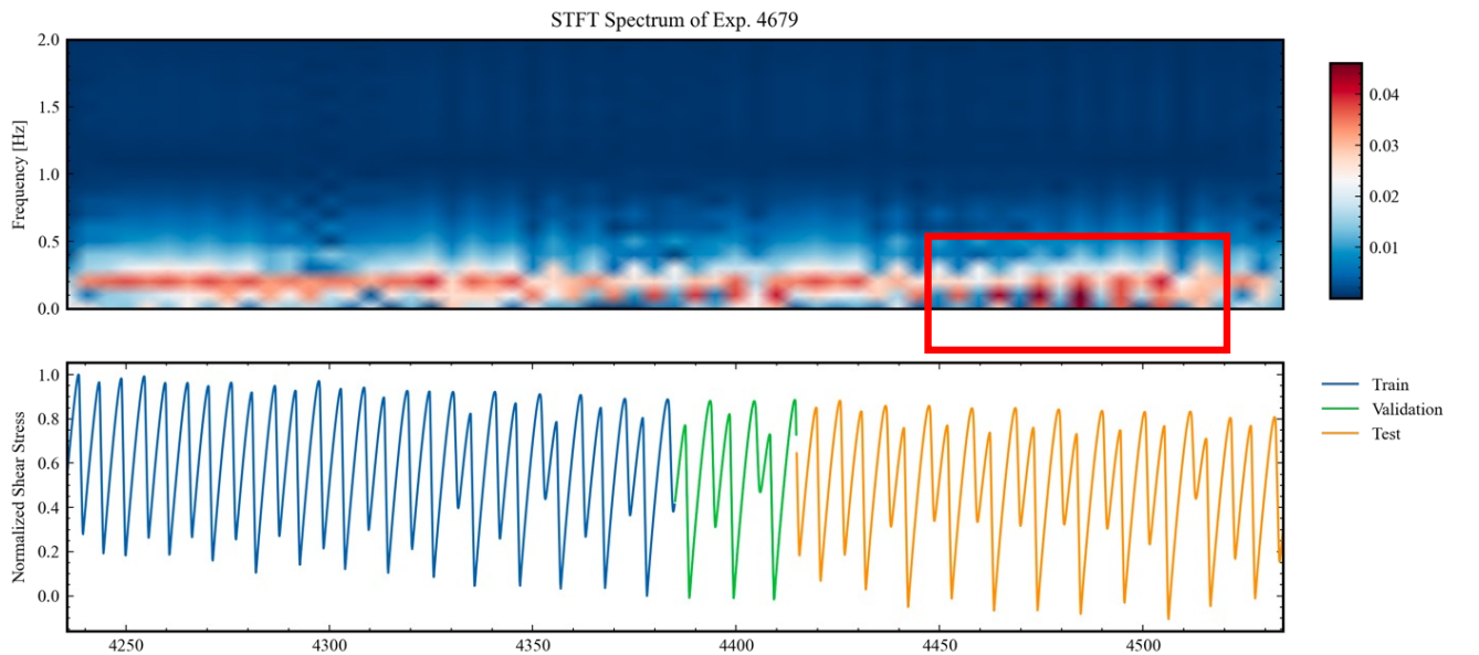
Figure 13. Short-Time Fourier Transform for Exp. 4679. Red box indicates the changes in frequency components in the test set.
