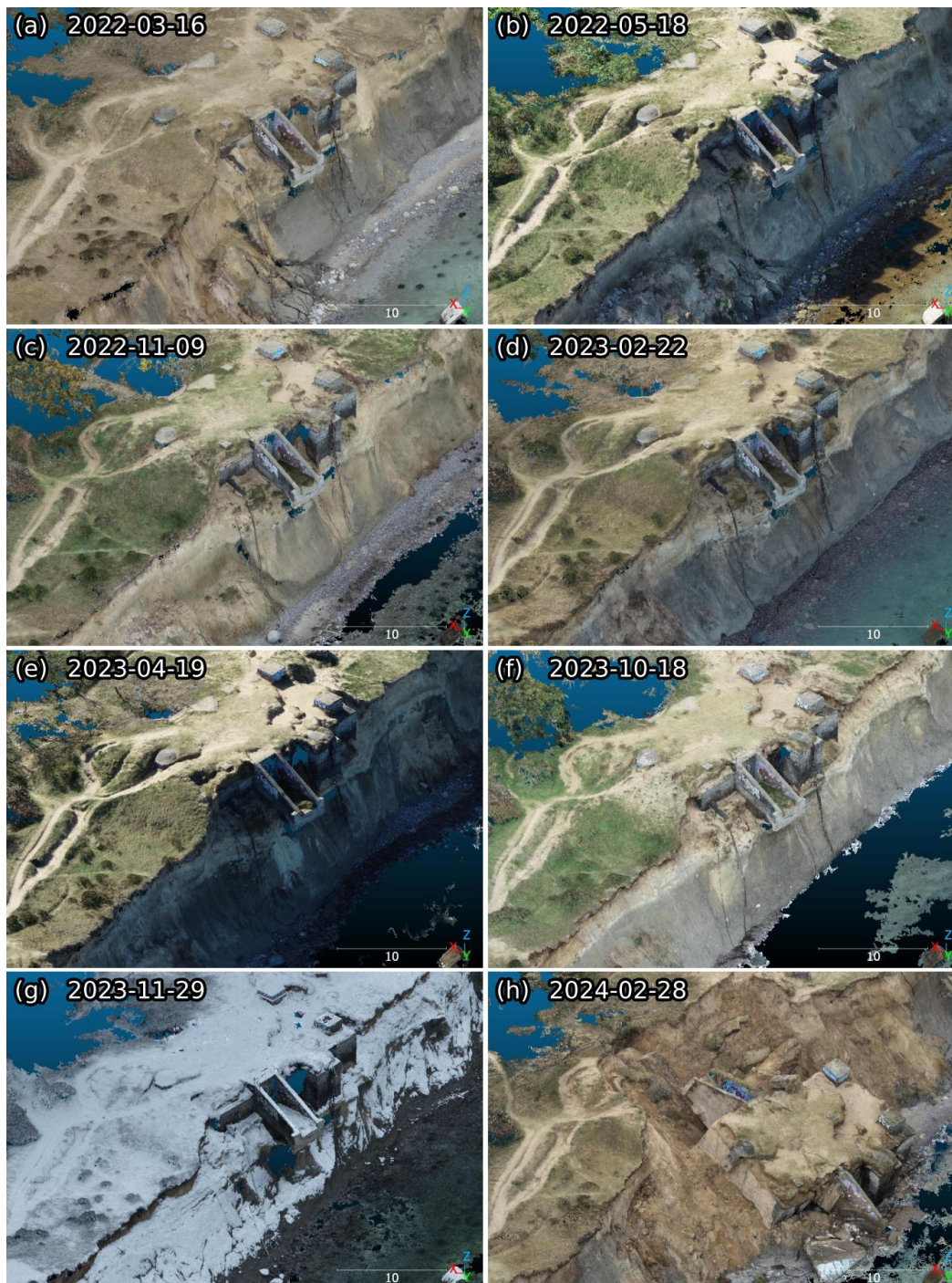
Figure 11. Point Clouds of the Bunker in the Wustrow study area from the northwest, generated with FACA Default parameters for field campaigns 1 to 8.
