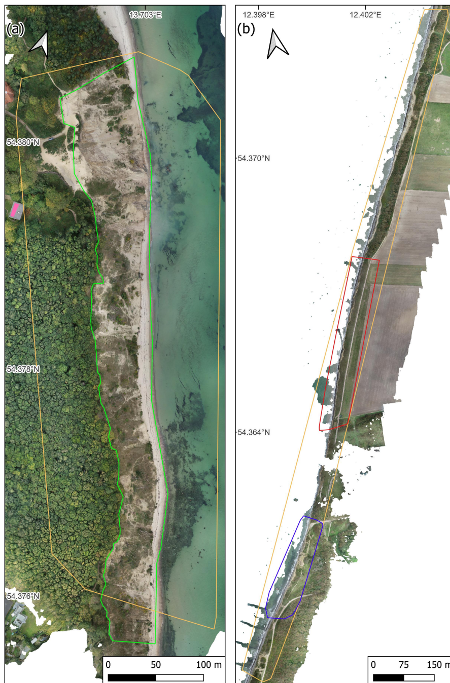
Figure 4. Orthophotos based on images from field campaign 6 with stable (pink filled polygon), sand cliff (green polygon), bunker area (blue polygon), coastal erosion area (red polygon) and the minimum bounding box (yellow polygons) of all images taken automatically on that day. (a) Sellin; (b) Wustrow.
