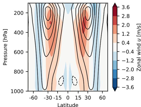
**Figure 8.** The time- and zonal-mean zonal wind for the slab control run (black contours) and the difference between the experiment with  $A = 40 \text{ W m}^{-2}$  and the slab control run (shading) for GFDL-AM2.
