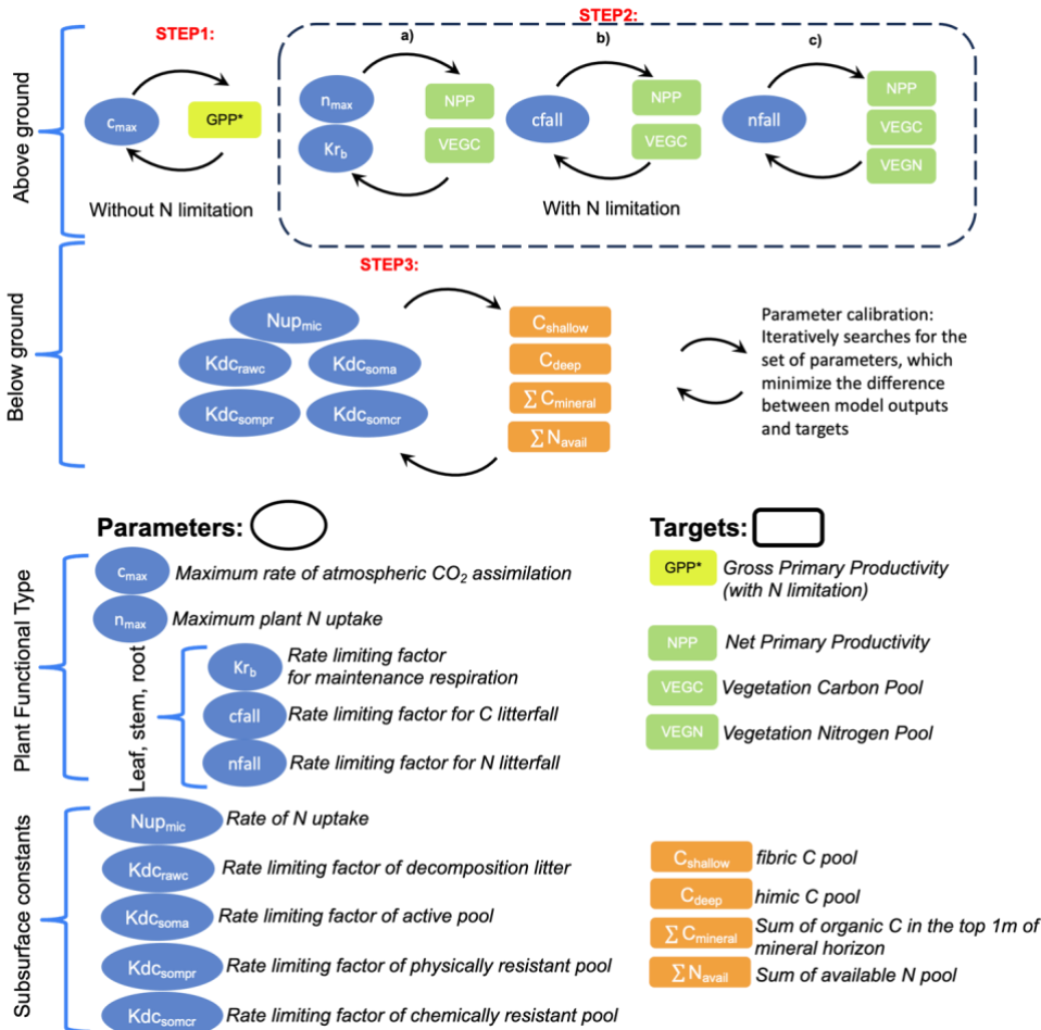
Figure 2. Schematics of the DVM-DOS-TEM model parameters and targets participated in the calibration process.
