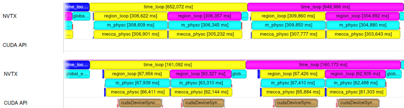
Figure 12. Example of an NVTX tracing with the Nvidia NSight System tool for the DWARF integration of the MIM chemical mechanism. Visualised are two subsequent time steps including the call of the kinetics integration: upper panel - CPU only, lower panel - kinetics integration on GPUs.
