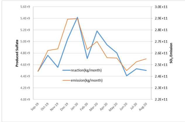
Figure 9: monthly sulfate from reactions (orange line, primary axis) and SO 2 emissions (blue line, secondary axis) in the GEFS-800 Aerosols simulation (kg/month).
