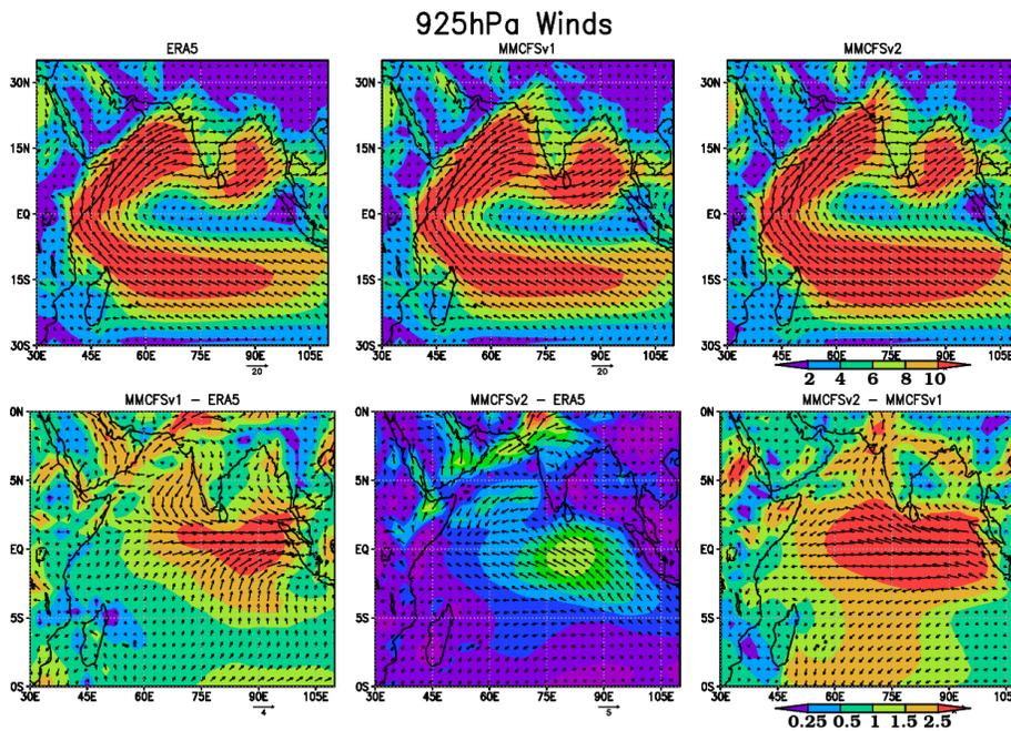
Figure 1b. 925hPa winds (vectors and shaded magnitude) from (a)ERA5 (b) MMCFSv1 © MMCFSv2, and biases (d) MMCFSv1 – ERA5 (e) MMCFSv2 – ERA5, difference between the model winds (f) MMCFSv2 – MMCFSv1
