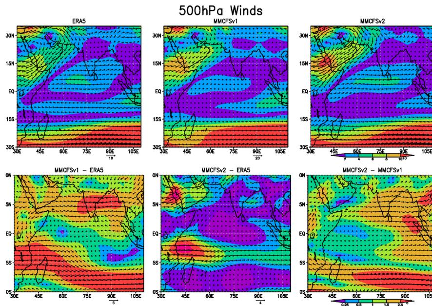
Figure 1d. 500hPa winds (vectors and shaded magnitude) from (a)ERA5 (b) MMCFSv1 © MMCFSv2, and biases (d) MMCFSv1 – ERA5 (e) MMCFSv2 – ERA5, difference between the model winds (f) MMCFSv2 – MMCFSv1
