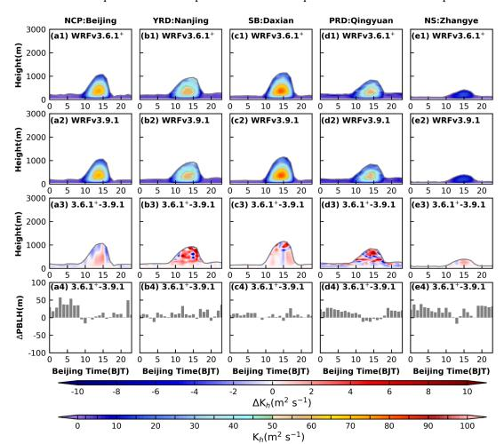
Figure 16. Time-height cross sections of heat turbulent diffusion coefficient (TDC) simulated by
