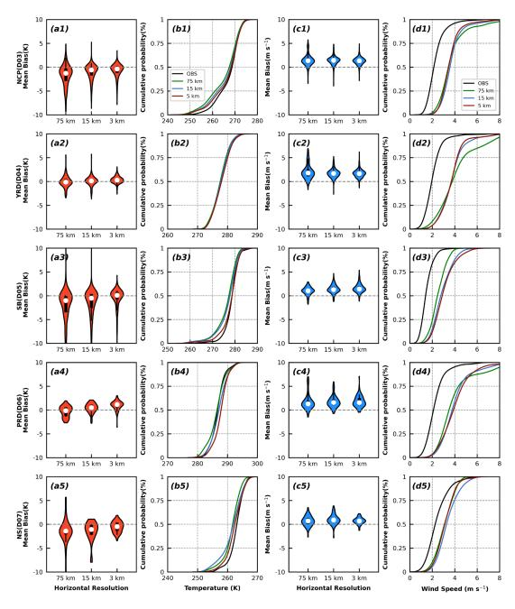
Figure 4. Violin-plots of mean bias of observed and simulated (a1-a5) 2-m temperature and (c1-c5) 10-m wind speed at different horizontal resolution (i.e., 75 km, 15 km, 3 km), cumulative probability of observed and simulated (b1-b5) 2-m temperature and (d1-d5) 10-m wind speed at different horizontal resolution (i.e., 75 km, 15 km, 3 km) for five regions.
