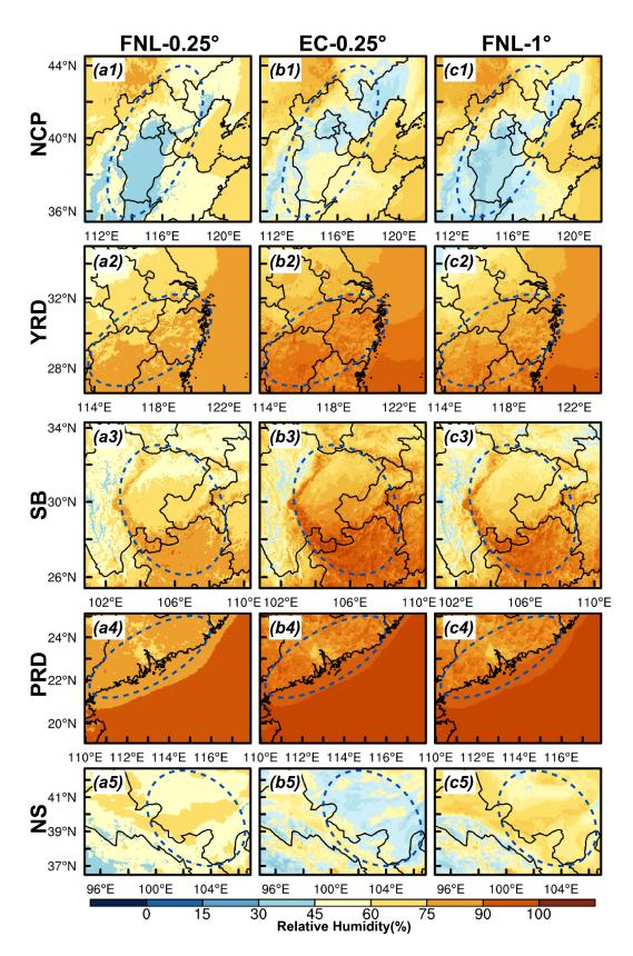
Figure 13. Regional distribution of 2-m relative humidity simulated by the (a) FNL-0.25°, (b) EC-0.25° and (c) FNL-1° for five regions in January, and the blue dashed circles indicate the regions where the results of the three experimental simulations differ significantly.
