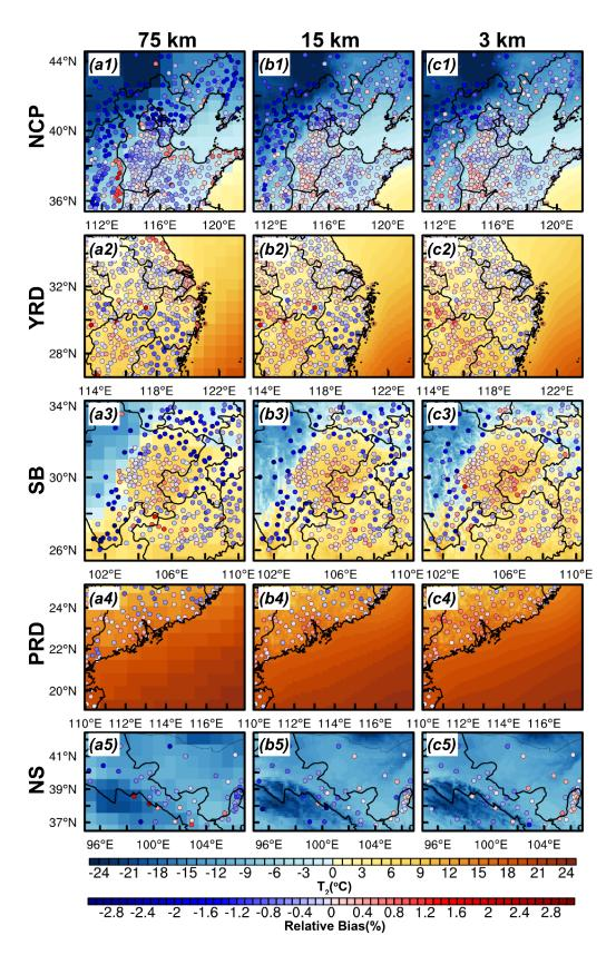
Figure 2. Regional distribution of 2-m temperature simulated by the (a) domain 1 (75 km), (b) domain 2 (15 km) and (c) domain 3 (3 km) for five regions in January, and distribution of relative bias between simulations and observations is denoted by scatters.
