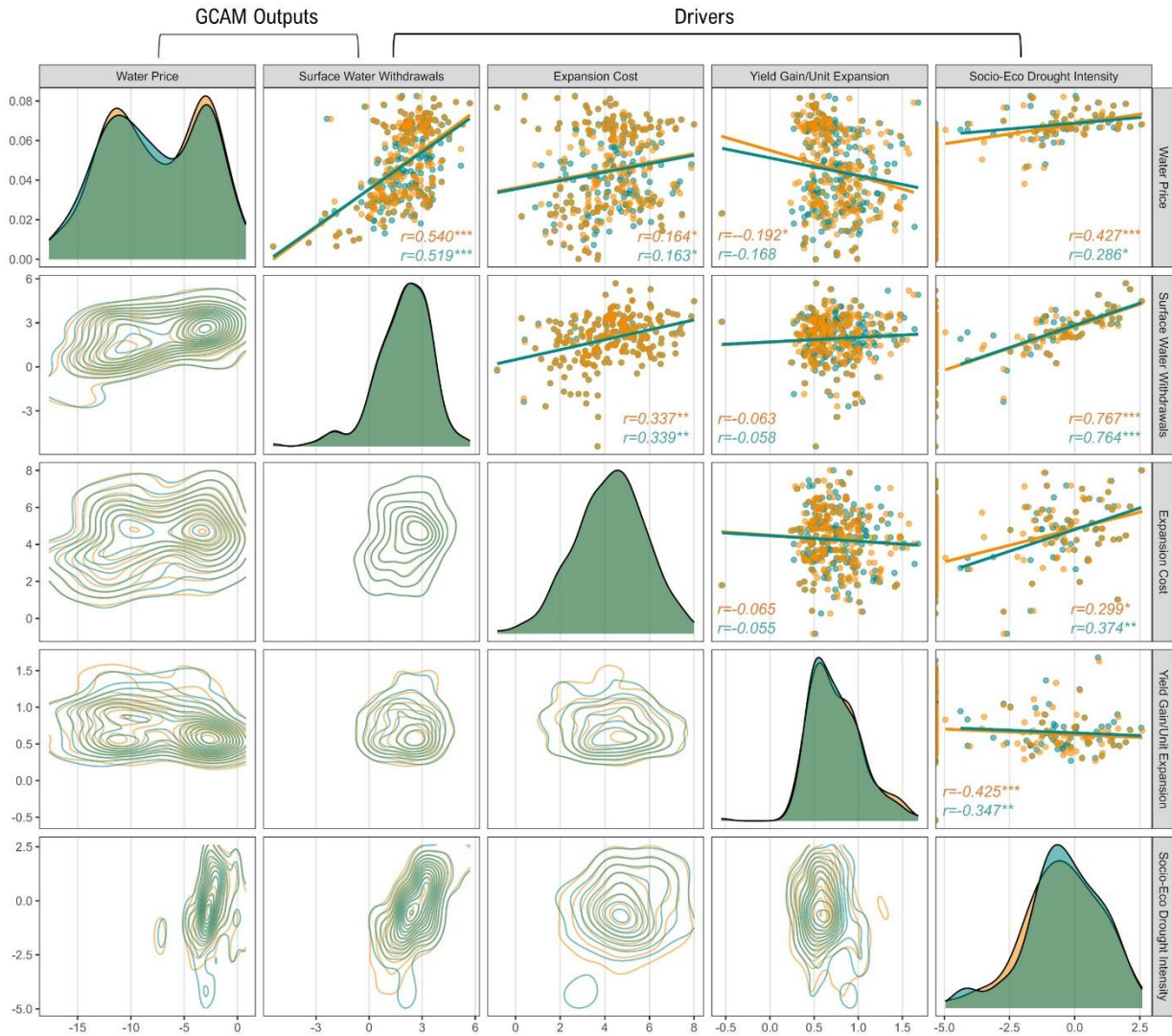
905 Figure 11. Paired density plots (lower half) and Pearson correlation plots (upper half) among drivers and GCAM outputs in 2050 under Feedbacks and No Feedbacks scenarios for selected basins. Drivers include cost for incremental expansion storage, median 910 water gain per unit storage capacity expansion at GCAM solved supply level, and socioeconomic drought intensity. GCAM outputs include water prices and water withdrawals (or demands). The orange and blue colours denote Feedback and No Feedback scenario, respectively. The asterisks next to the level of correlation (e.g., three asterisks mean strong correlation). Basins are included for the linear regression for water gain per unit expansion and socioeconomic drought intensity if the water supply is above the maximum natural yield and there is a deficit between sub-annual demand and natural runoff. The maximum natural yield is the amount of natural water that can be provided without any reservoir regulation. All variables are normalized with log transformation and both axes are unitless.
