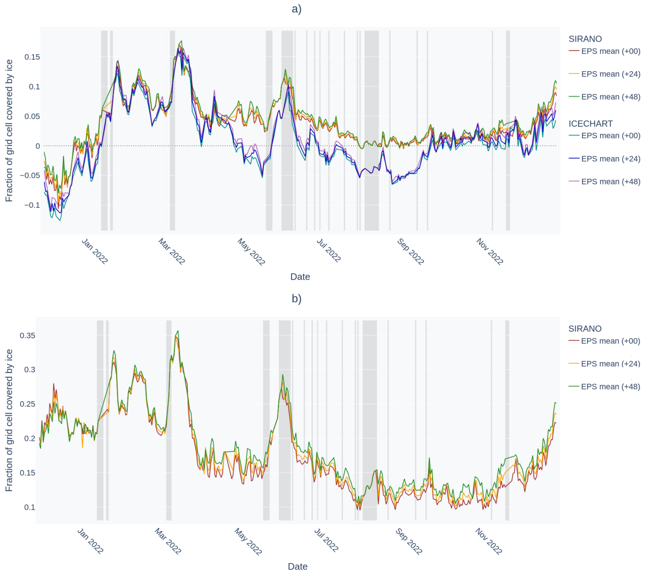
Figure 8. Time evolution of (a) RMSE and (b) ME for SIC based on daily comparison of model values in various forecast ranges averaged over the entire model domain. Differences are shown for comparison with the passive microwave SIC product that is assimilated (SIRANO) and for a comparison with subjective ice charts that are produced by ice analysts. Shaded intervals mark model cycles when no data was assimilated.
