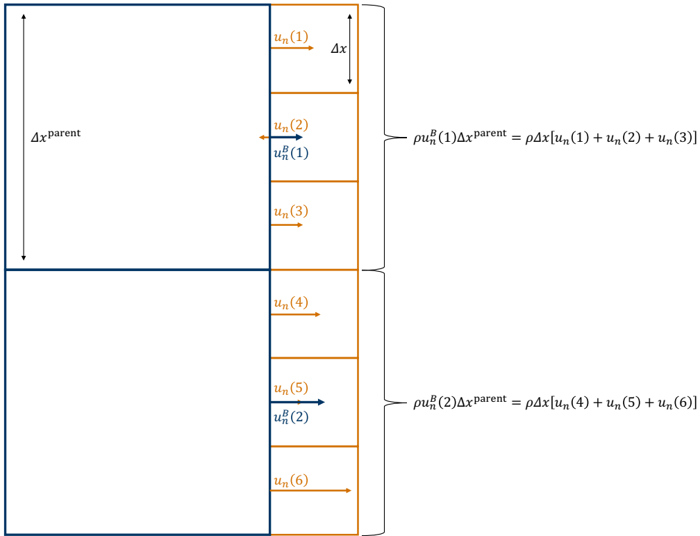
Figure 1. 2D illustration of a nested setup in which the integration length scales are set to the gridsize of the parent model. In this setup the mass flux through a parent cell (blue) at the boundary of the child model (brown) is conserved, while the child model is free to generate turbulence on smaller scales.
