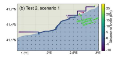
• The example above shows alongshore current close to the coastline in an area where the low-resolution CMEMS grid applies. The resolution of 2.5 km in these areas mean that such coastal processes are not resolved hydrodynamically anyway. Therefore it would be very unlikely for particles to reach the real coastline that would otherwise be caught in a current resulting from a coastal process where low-resolution hydrodynamic data applies.
