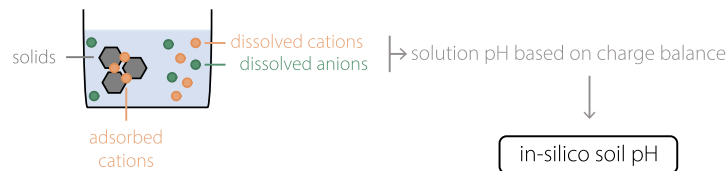
Figure 1: Schematic of soil pH calculation procedure. After a field simulation is run to represent a specific field soil (Step 1), in-silico field data are obtained (Step 2) for the concentrations of solid phases (left), adsorbed cations (middle) and dissolved cations and anions (right). In Step 3, sampled in-silico field data are converted to input data for a laboratory simulation in which extractable/exchangeable cations/anions are converted to a combination of salt/oxide phases to be added to the laboratory beaker/flask with additional phases depending on the extractant (or buffer) solution. In Step 4, these added phases are dissolved in the laboratory beaker/flask to reach equilibrium, after which the calculated solution pH corresponds to soil pH ( pH_s ) of the in-silico field soil in Steps 1 and 2.
