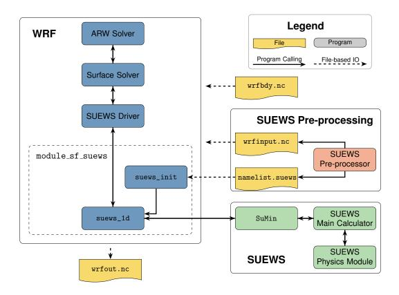
**Figure 2.** WRF-SUEWS system consists of the new |module\_sf\_suews| added into WRF (blue) to interact with SUEWS via |SuMin| (green) using input files pre-processed by SUEWS pre-processor (yellow). File-based input/output flow (dashed) and runtime calling logic (solid lines) are shown.
