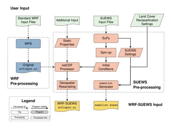
**Figure 3.** Workflow for WRF-SUEWS pre-processing system (WSPS)
