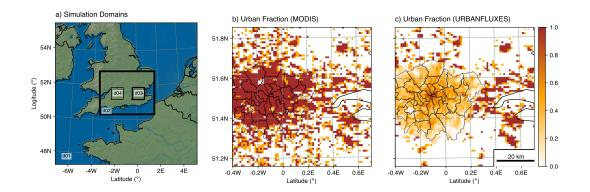
**Figure 5.** Model domain configurations: (a) four simulation domains (d01-d04) and urban land cover (paved and buildings) fraction in d03 (1 km resolution) based on (b) the WRF default MODIS dataset and (c) updated information for Greater London from URBANFLUXES project (Lindberg et al. 2020). The land cover information is accessible in Sun et al. (2023a).
