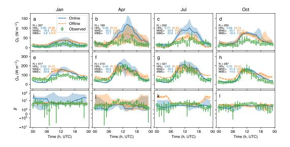
Figure 13. Diurnal pattern of simulated (median: online - line, offline - dashed; IQR: shading) and observed (median: circle, IQR: vertical line) fluxes: (a-d) sensible  $(Q_H)$  and (e-h) latent  $(Q_E)$  heat fluxes, and (il) Bowen ratio  $(\beta = Q_H/Q_E)$  (hourly median) for (columns) four two-week periods in different seasons (Table 4) at KCL. Metrics defined in Sect. 3.3
