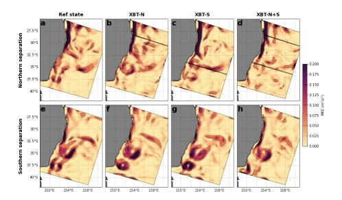
**Figure 9.** The surface MKE is compared between the (a) Reference state, (b) XBT-N, (c) XBT-S and (d) XBT-N+S for the case when the EAC is in a northern separation phase. For the southern separating EAC phase, the surface MKE is compared between the (e) Reference state and the (f) XBT-N, (g) XBT-S, (h) XBT-N+S. Black lines in panels b-d indicate location of the XBT lines.
