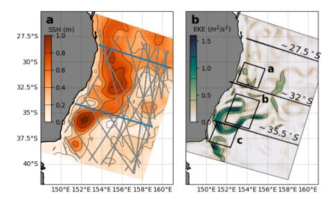
**Figure 3.** Snapshots of model conditions with examples of observations and analysis regions. (a) A snapshot of SSH (colour map) is shown with a single 5-day cycle of SSH (grey dots) and XBT (blue dots) observations. (b) A snapshot of EKE (colour map) is shown, with boxes and lines showing key regions and diagnostic transects used in the analysis.
