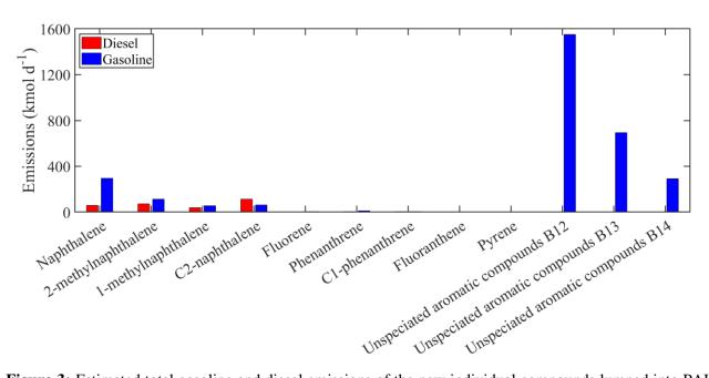
**Figure 3:** Estimated total gasoline and diesel emissions of the new individual compounds lumped into PAH1 for Europe.
