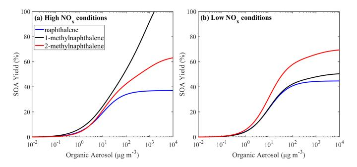
**Figure 9:** Estimated SOA yields of naphthalene, 1-methylnaphthalene and 2-methylnaphthalene under (a) high NOx and (b) low NO<sub>x</sub> conditions. The curves are generated using the estimated parameters of Table S2.
