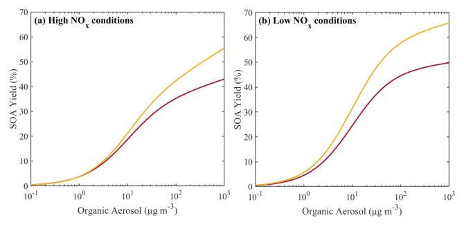
**Figure 10:** Estimated aerosol mass fractions of the new lumped PAH species under (a) high  $NO_x$  and (b) low  $NO_x$  conditions. The yield curves are generated using the mass-based yields of Table 3.
