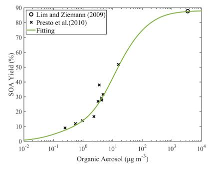
Figure 7: Estimated SOA yields of n-Heptadecane under high NOx conditions. The curve is generated using the estimated ai (0.0771, 0.024, 0.6291, 0.1506 and 0). The data from the studies of Lim and Ziemann (2009) and Presto et al. (2010) that were used by the simplified algorithm are also shown.
