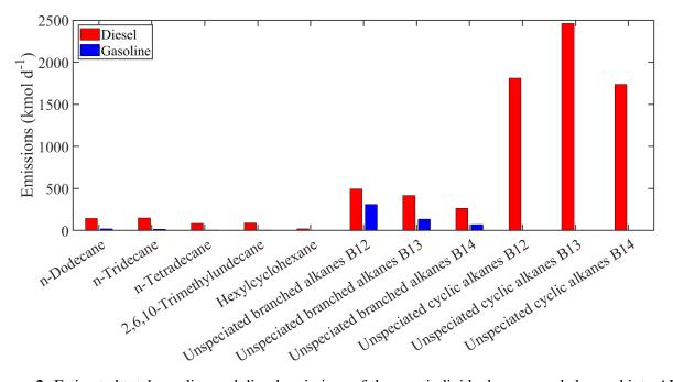
**Figure 2:** Estimated total gasoline and diesel emissions of the new individual compounds lumped into ALK6 for Europe
