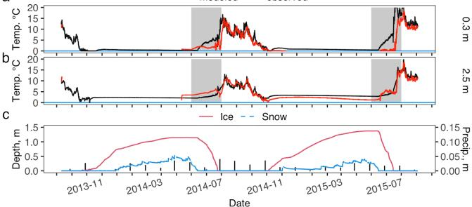
Figure 1. Atqasuk modeled and observed lake water temperature at 0.3 m (a) and 2.5 m (b) and modeled lake ice depth, lake snow depth and measured monthly precipitation (vertical black bars) (c). Gray shading indicates periods of uncertainty in temperature sensor depth when ice-rafting may have moved the sensor to shallower water. The y-axis of panel (a) is limited to water temperatures > 0 °C as the LAKE model water temperature is limited to > 0 °C.
