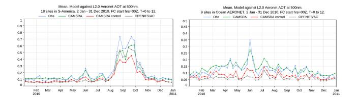
**Figure 9**. Evaluation of total AOD at 550 nm from OpenIFS/AC against observations from AERONET at 500 nm. Also results from the CAMS reanalysis, and its control experiment are included for reference.
