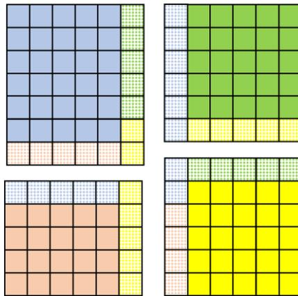
**Figure 2. Example of halo regions corresponding to the parallel decomposition in Fig. 1. Spotted boxes around each subdomain denote each process's halo region; the color of each spotted box indicates the corresponding source process.**
