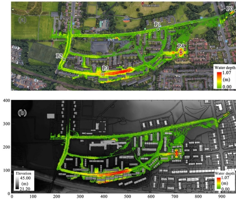
520 Figure 7: Flood inundation extent at t=4200s calculated by (a) dg2 solver and (b) the improved SGC solver. Background map in (a) are © Google Maps screenshot(s).
