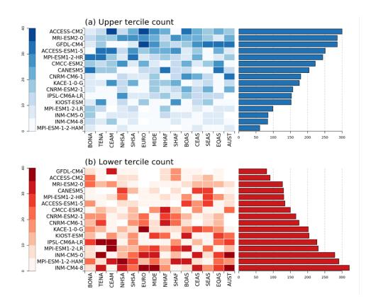
Figure 9: (a) Counts of the number of times that each CMIP6 model is ranked in the upper tercile (top 5) across all 7 CFWIS components and 3 x 2 skill metrics (correlation, RMSE, and ratio of standard deviation for the mean and 90<sup>th</sup> percentile). The grid (left) shows the breakdown of total counts for each of the 14 GFED regions. The bars (right) indicate the total count across all regions. (b) As (a) but for the lower tercile (bottom 5).
