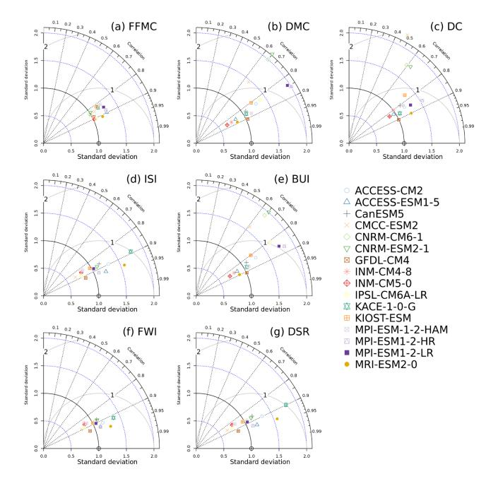
280 Figure 5: Taylor diagrams showing the capacity of 16 CMIP6 models to simulate annual means in the seven CFWIS indices. The correlation coefficient is plotted in relation to the polar axis, the normalised RMSE in relation to the internal circular axis, and the normalised standard deviation in relation to the horizontal axis. GEFF-ERA5 is represented by an empty dot on the horizontal axis.
