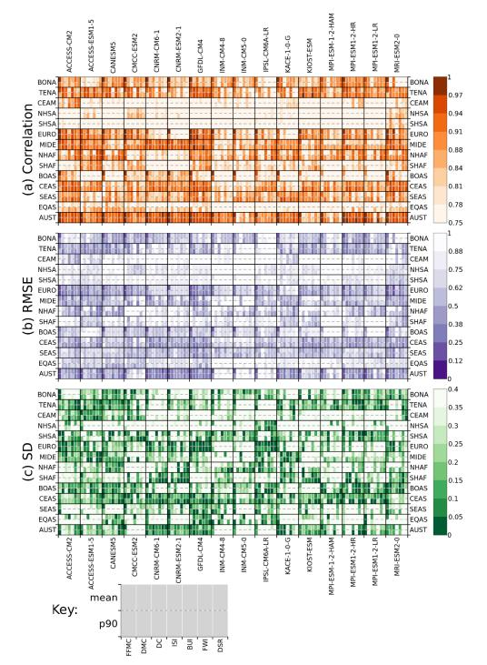
Figure 7: Individual CMIP6 model (a) correlation, (b) RMSE and (c) absolute log of the ratio of standard deviation with respect to GEFF-ERA5 for the fire season mean and 90<sup>th</sup> percentile across each of the seven CFWIS indices and each of the 14 GFED fire regions. Darker colours show higher spatial correlations, and lighter colours lower. The fire season for each region is defined as those months for which the average burned area is greater than 50% of the monthly maximum (see Fig. 4).
