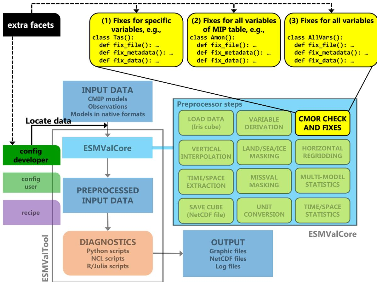
**Figure 1.** Schematic representation of ESMValTool. Non-transparent colors correspond to elements that have been altered/added to allow CMOR-like reformatting of native model output during runtime, which is included into ESMValTool as part of the preprocessing chain. Adapted from Righi et al. (2020).
