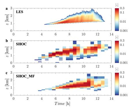
Figure 7: Time-height plot of (a) LES, (b) SHOC, (c) SHOC+MF cloud fraction for the ARM shallow cumulus case. The LES cloud fraction corresponds to the cloud sampling definition (i.e.,  $q_l > 1 \times 10^{-5} \text{ kg kg}^{-1}$ ). Cloud fraction values < 0.001 are masked and not plotted here.
