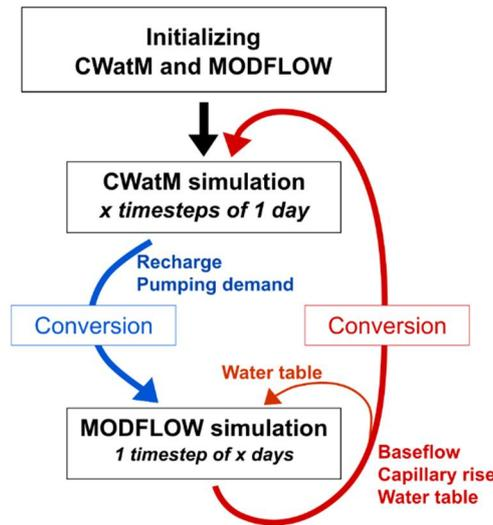
**Figure 2: Scheme of the CWatM-MODFLOW coupling. Conversion refers to changing spatial resolution and units and passing to MODFLOW model using BMI (blue case) or reading MODFLOW output (red case). Note MODFLOW model can be used at different space and time resolutions**
