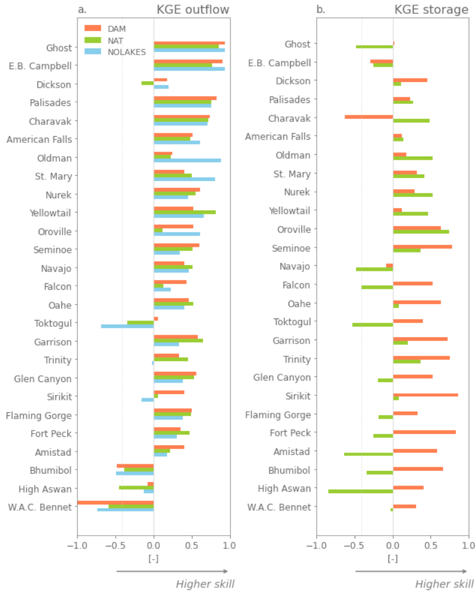
Figure 3. Evaluation using Kling-Gupta Efficiency (KGE) of the (Hanasaki et al., 2006, ; DAM) and (Döll et al., 2003, ; NAT) parametrizations with observed inflows, and using inflow as outflow (assuming there is no lake; NOLAKE) against observed outflow (panel a) and observed storage (panel b) using observations from Yassin et al. (2019). The reservoirs are ordered from low to high capacity ratio, defined as the ratio between the mean annual inflow and storage capacity (see Table A2).
