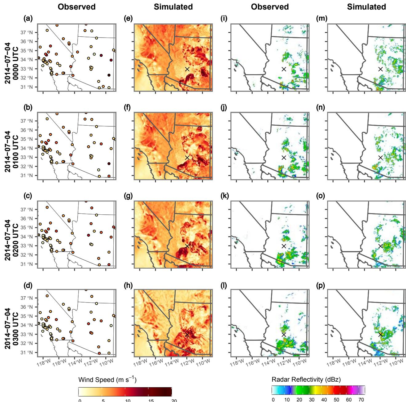
**Figure S1:** (a)-(d) Observed ASOS wind speed, (e)-(h) simulated wind speed, (i)-(l) NEXRAD composite radar reflectivity, and (m)-(p) simulated radar reflectivity for 4 July 2014, 0000-0300 UTC. The black  $\times$  marks the location of Phoenix, Arizona.
