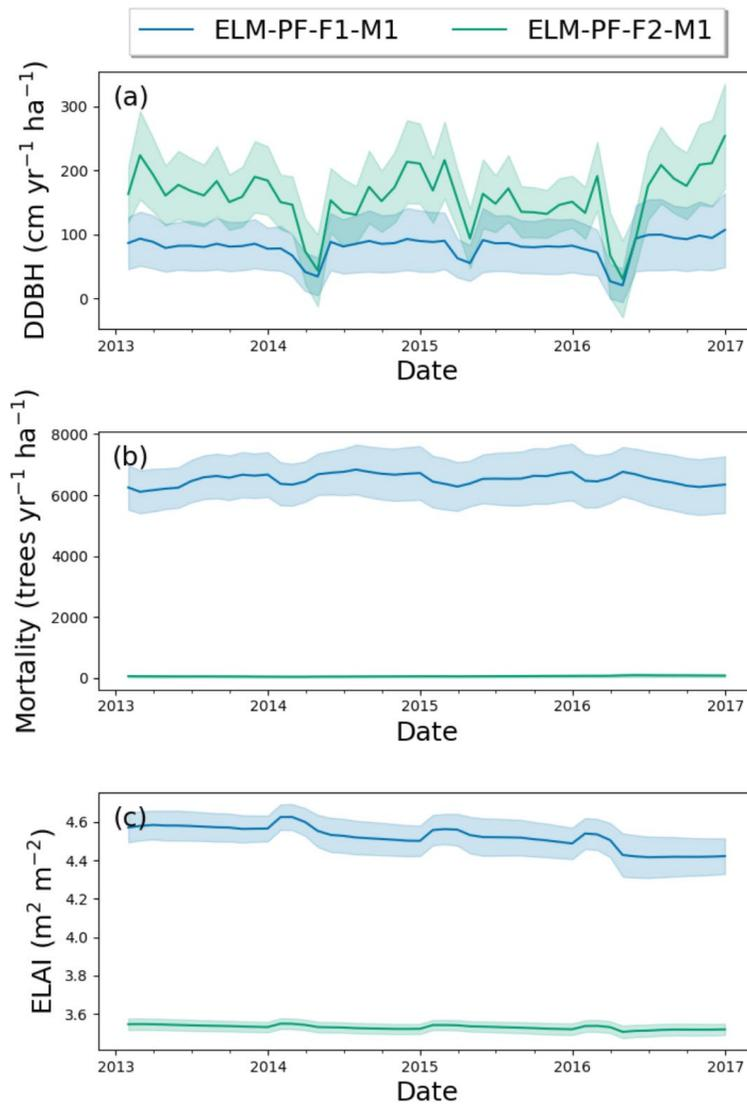
**Figure R2.** Growth (increment of diameter at breadth height, DDBH) (a) vs. mortality (b), and exposed leaf area index (c) for ELM-PF-F1-M1 and ELM-PF-F2-M1. Solid line is spatial average and shaded area is the standard deviation over the simulation domain.
