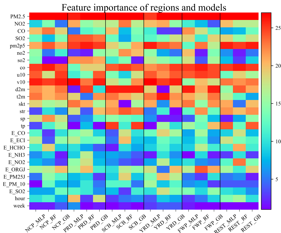
Figure 5. Heatmap of empirical features for six regions with three machine learning models. Each column represents the rearrangement of the sum of 15 monitoring stations and 4 prediction horizons. Black vertical lines are used to distinguish each region. The warmer the row color, the more critical the corresponding feature.
