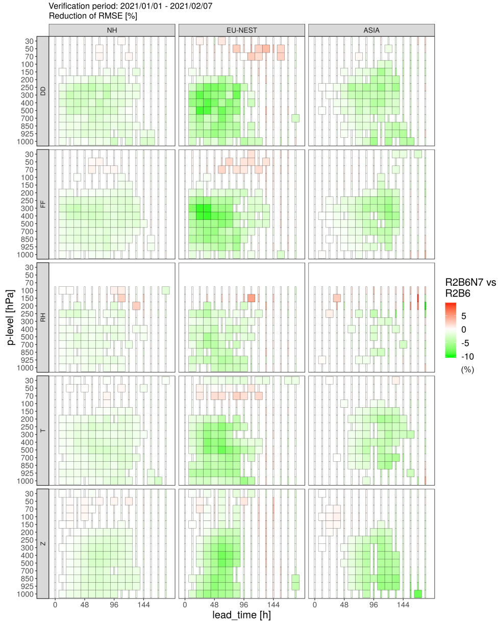
Figure 14. Scorecard for verification against radiosonde ascents for wind direction (DD), wind speed (FF), relative humidity (RH), temperature (T) and geopotential (Z) in the same regions as in Fig. 12. Colours indicate relative RMSE differences (%) between R2B6N7 and R2B6, and wide boxes indicates statistical significance at the 95%-level.
