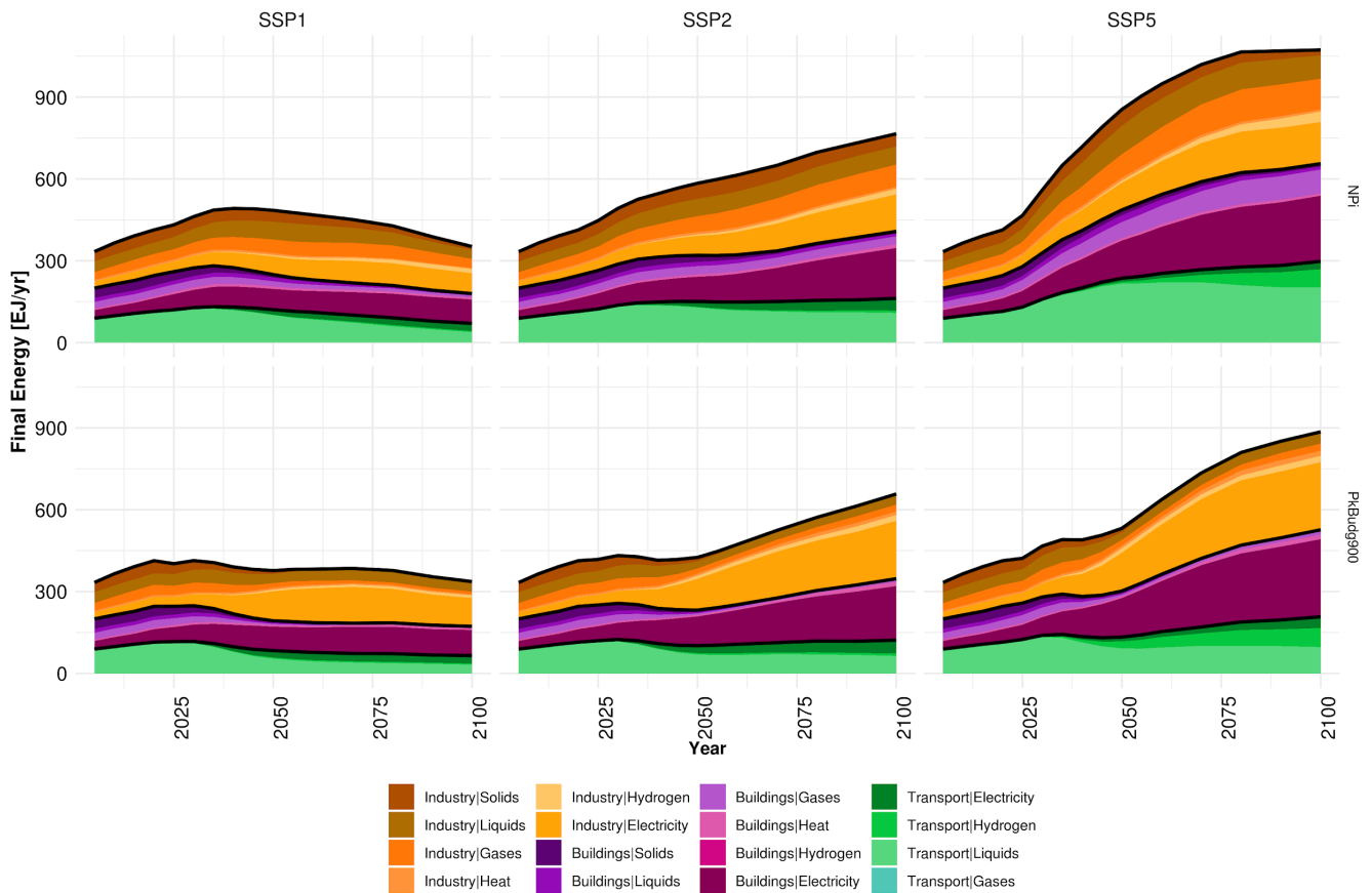
Figure 8: Final energy mixes for sectors by carrier for the NPi and pkBudg900 (1.5°C) scenario of SSP1, SSP2 and SSP5
