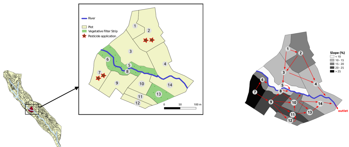
Left: portion of La Morcille catchment selected to perform sensitivity analysis. Yellow units stand for vineyard plots while green units stand for vegetative filter strips. Brown stars denote locations of pesticide application. Right: slopes and connections between elements.
