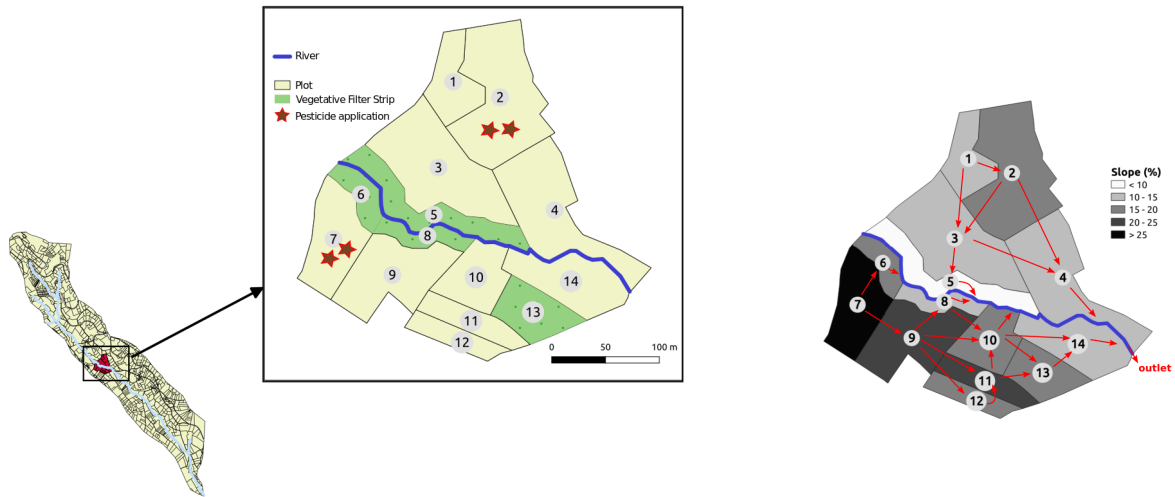
Figure 1. Left: portion of La Morcille catchment selected to perform sensitivity analysis. Yellow units stand for vineyard plots while green units stand for vegetative filter strips. Brown stars denote locations of pesticide application. Right: slopes and connections between elements.
