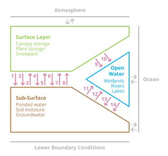
**Figure 1.** Schematic blueprint of the terrestrial water cycle featuring the three components 'Surface Layer', 'Sub-Surface', and 'Open Water', their transfers of information as numbered arrows (see Table 1), and their relationships with external models (atmosphere and ocean).
