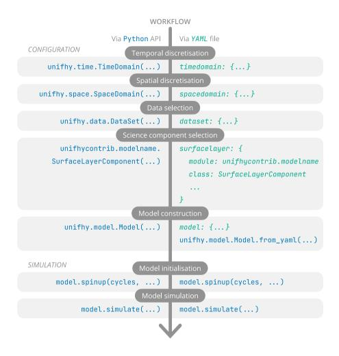
**Figure 3.** Workflow to follow to configure and use the modelling framework, exclusively via the Python API on the left-hand side, and via the use of a YAML file for configuration on the right-hand side.
