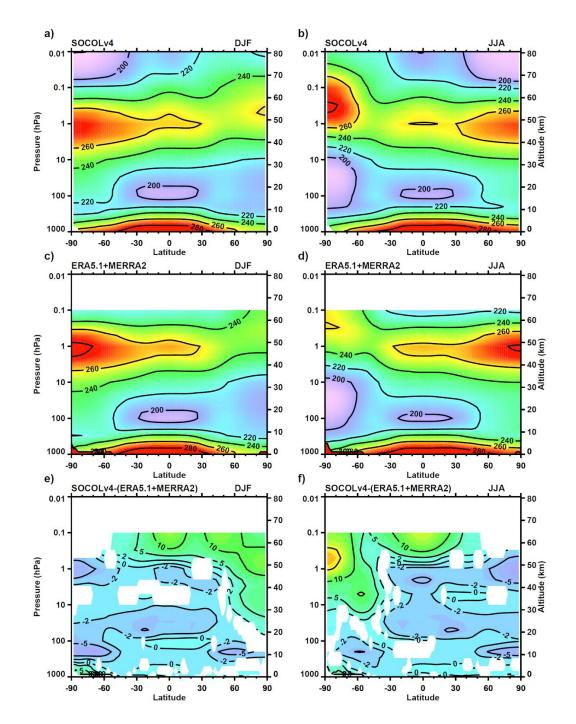
Figure 6. Zonal mean temperature climatology for DJF (left panel) and JJA (right panel) simulated with SOCOLv4 (a, b), mean of ERA5.1 and MERRA-2 reanalysis (c, d) and differences between simulated and reanalysis data (e, f). Contour intervals for the differences are -30, -20, -10, -5, -2, 0, 2, 5, 10, 20, 30, 40 K. White places denote regions where the difference between model and reanalysis data is not statistically significant at 95% confidence level.
