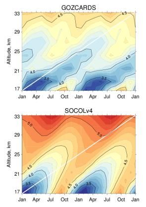
Figure 9. Annual cycle of water vapor mixing ratio (ppmv) averaged between 15°N and 15°S and over 1991-2012 for the GOZCARDS satellite composite (upper panel) and SOCOLv4 (lower panel). Two consecutive cycles are shown. The white line in both panels indicates the approximate slope of the GOZCARDS tape recorder signal.
