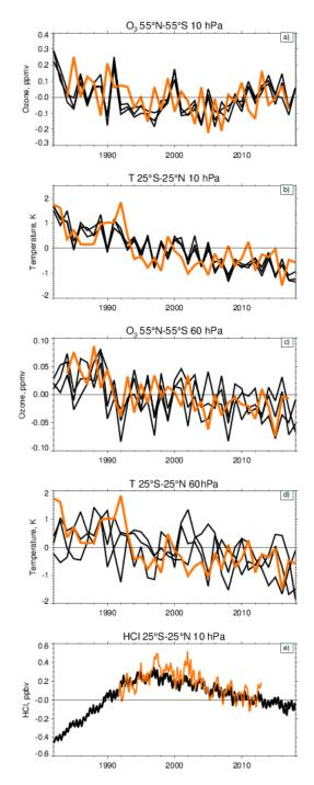
Figure 16. (a and c): Near global (55°S-55°N) annual mean ozone evolution at 60 and 10 hPa compared to the BASIC composite. (b and d): Tropical annual mean evolution of temperature at 60 and 10 hPa compared to ERA5. (e): tropical monthly mean (smoothed with the 3-month running mean) evolution of HCl at 10 hPa compared to the GOZCARDS composite. Black lines: three model ensemble members. Orange lines: observations.
