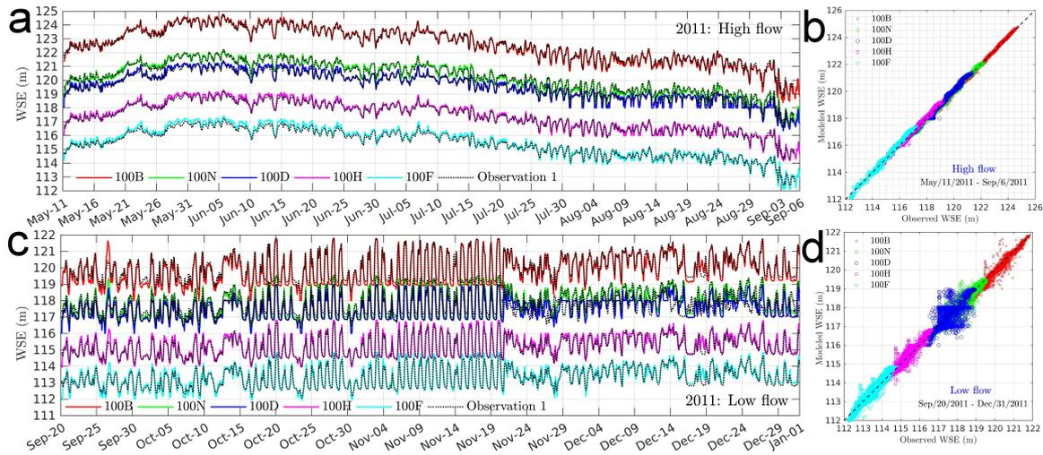
**Figure 6.** The comparison of water surface elevation from model and observations during high flow and low flow in 2011. (a-b) Hourly recorded time series of WSE and 1:1 plot during high flow. (c-d) Hourly recorded time series of WSE and 1:1 plot during low flow.
