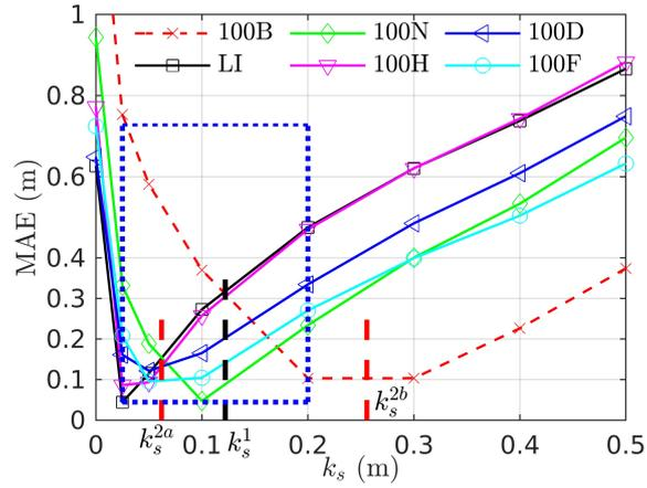
**Figure A3.** The variation of mean absolute error (MAE) between modeled and observed WSE at six locations using different roughness parameters. Black and red vertical lines represent the optimal roughness height using one-ks and two-ks strategy.
