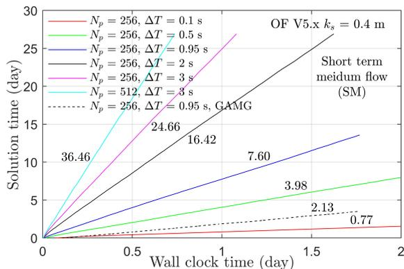
**Figure 13.** The advancement of solution time with respect to wall-clock time.  $N_p$  and  $\Delta T$  denote the number of processors and time step. Linear solver used for solid and dashed lines are DIC-PCG and GAMG, respectively. The line slope or the computational efficiency is denoted by the values adjacent to each line.
