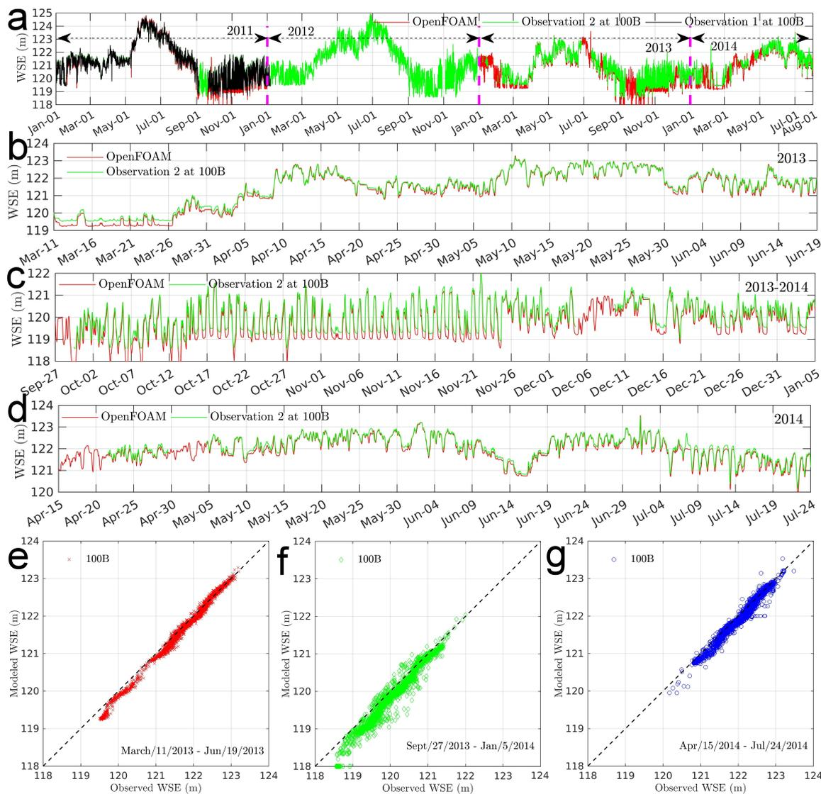
**Figure 9.** Medium-term model validation for water surface elevation. A comparison of hourly recorded WSE from model and observations during 2011-2014 (a), medium flow (b), low flow (c), and high flow (d). (e-g) denote the 1:1 plot during medium, low, and high flow scenarios.
