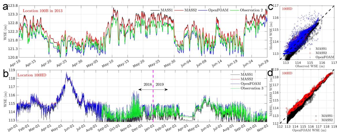
**Figure 12.** A comparison of water surface elevation (WSE) from MASS1, MASS2, OpenFOAM, and observations at 100B during 2013 (a) and at 100HD during 2018 - 2019 (b). (c) denotes the 1:1 plot of WSE between models and observation for 100HD; and (d) denotes that between OpenFOAM and MASS1/2. Details of the WSE from MASS1 and MASS2 can be found in (Niehus et al., 2014).
