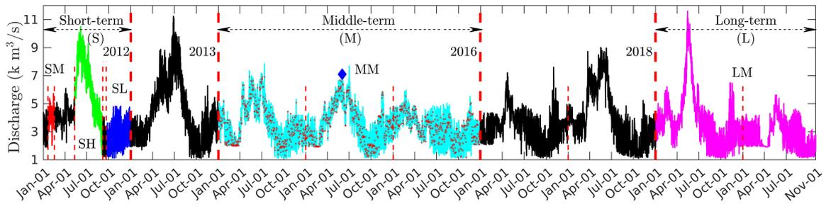
**Figure 4.** The time series of inlet flow rate during the years 2011-2019. S, M, and L denote short, medium, and long term. SM, SH, and SL denote the medium, high, and low flow in the short-term period; MM and LM denote mixed flow in the medium-term and long-term periods.
