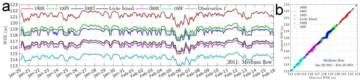
**Figure 5.** The comparison of water surface elevation between the model and observations using the calibrated roughness field (case OF in Table 1) during a medium flow in 2011. (a) An hourly recorded WSE and (b) a 1:1 plot.
