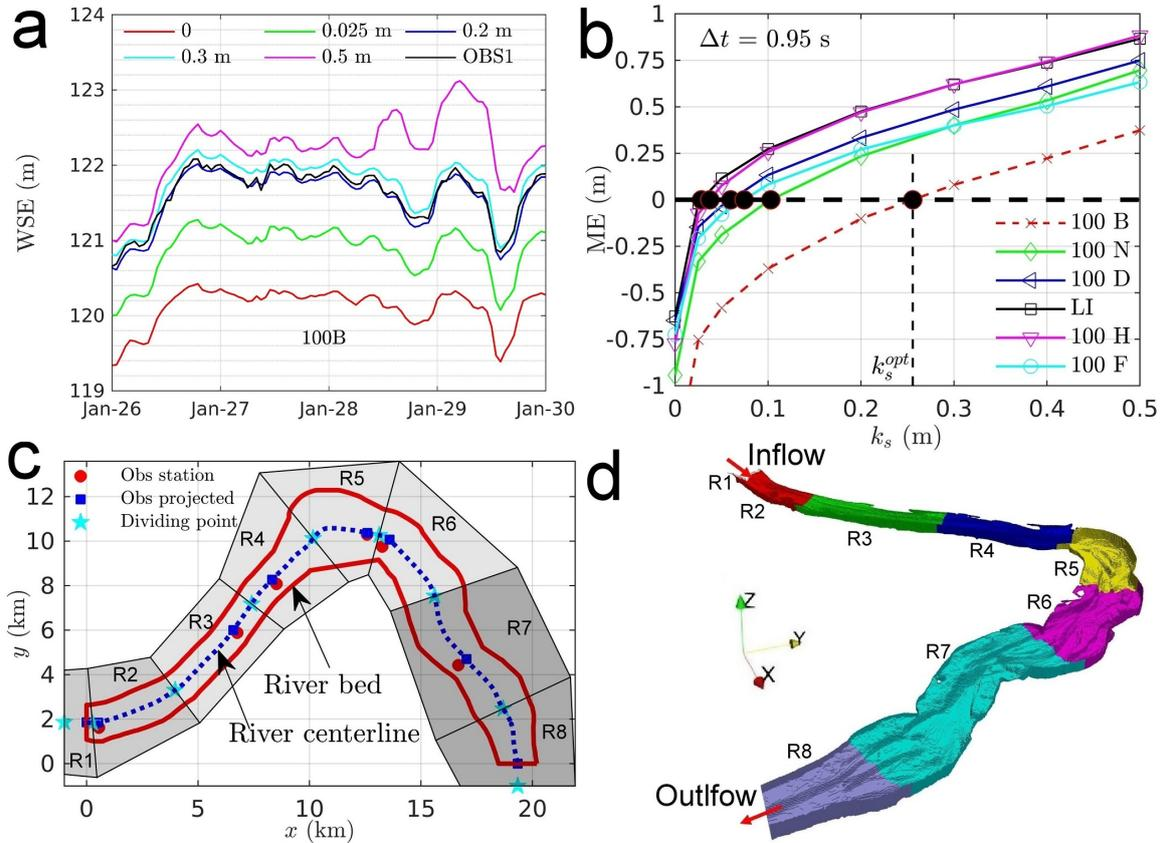
**Figure 3.** The effect of roughness height on WSE at a single location (a), ME between modeled and observed WSE at six locations (b), the procedure of generating eight roughness regions (c), and the 3D view of each region represented in mesh (d).
