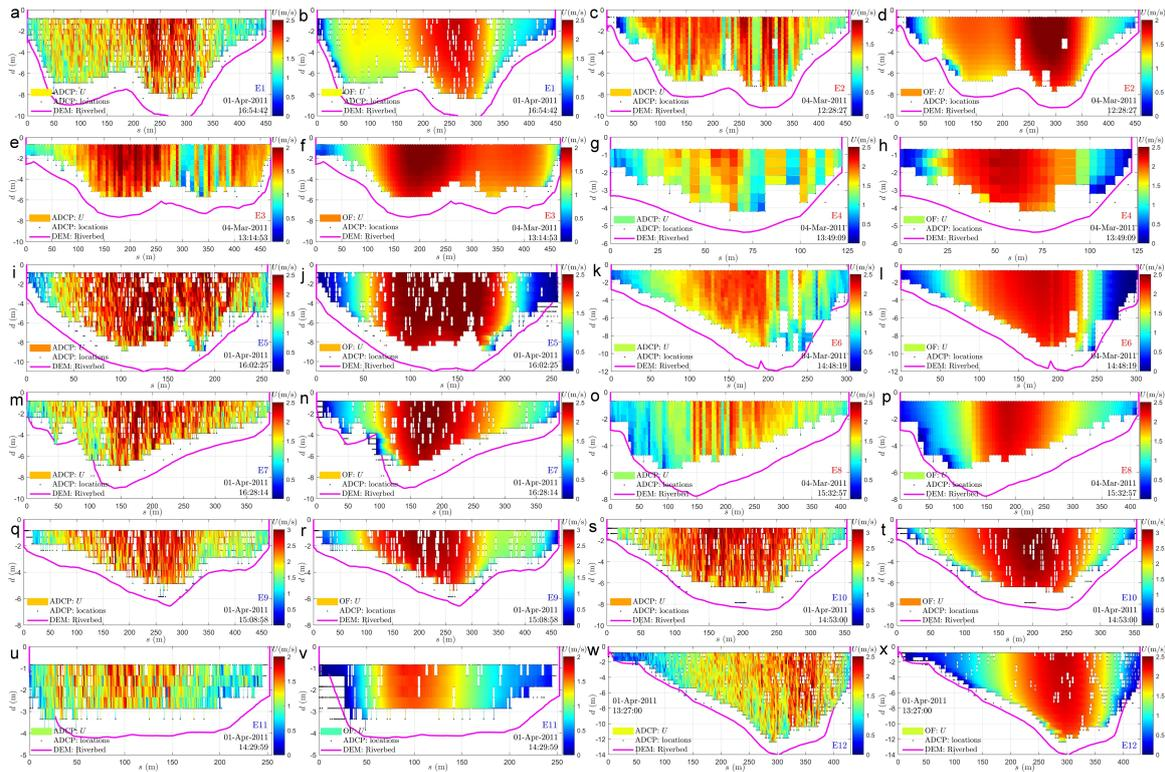
**Figure 7.** The velocity magnitude distributions on cross-section E1 - E12 from ADCP surveys (Columns 1 and 3) and CFD modeling (Column 2 and 4). Cross-section names (E1 - E12) with red and blue color denote survey dates on March-4 and April-1, 2011, respectively. Symbols  $d$  and  $s$  denote depth away from the water surface and distance from the right bank (see Figure 1c), respectively.
