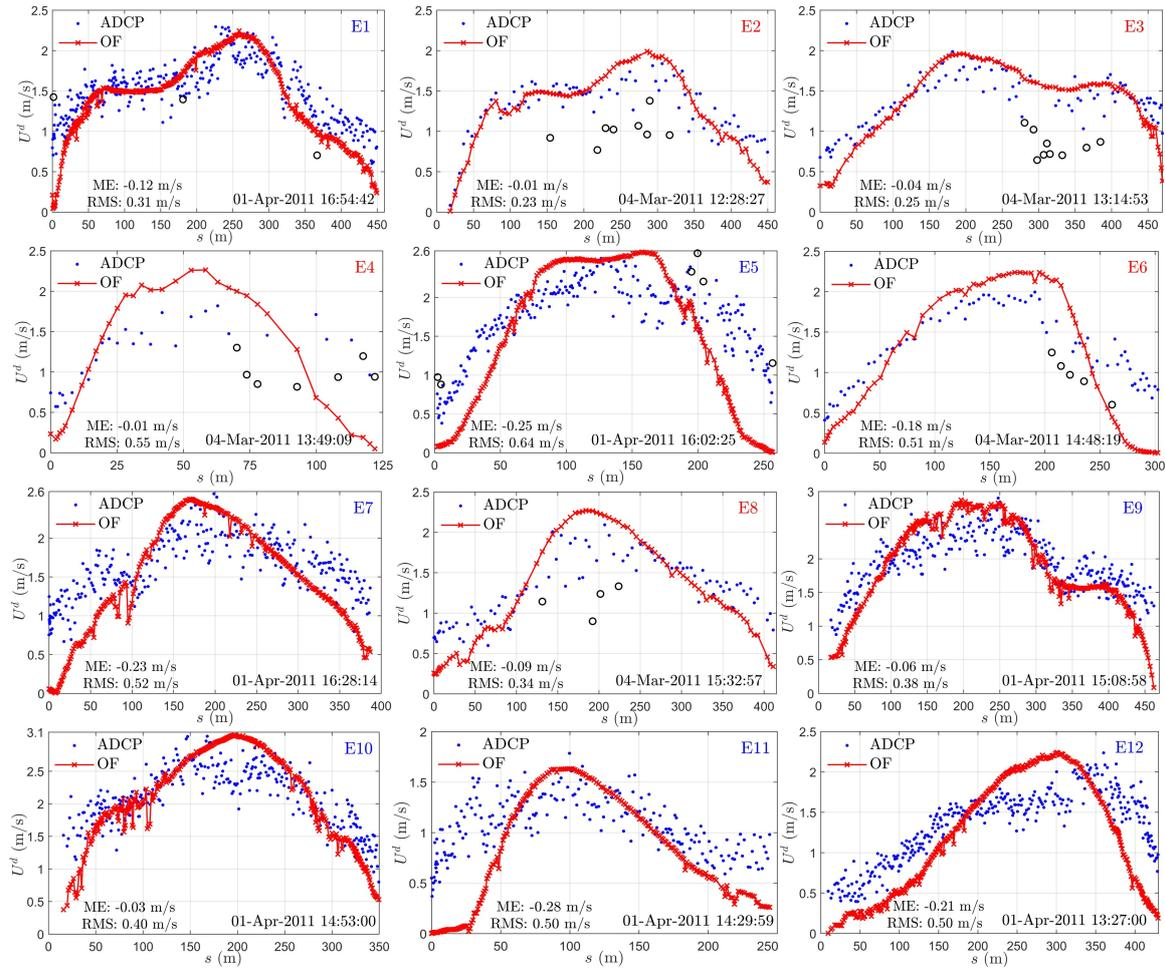
**Figure 8.** The comparison of depth-averaged velocity magnitude determined from ADCP surveys and CFD modeling. Black circles denote measured velocity outliers visually determined through velocity components (Figure A5 or A6).
