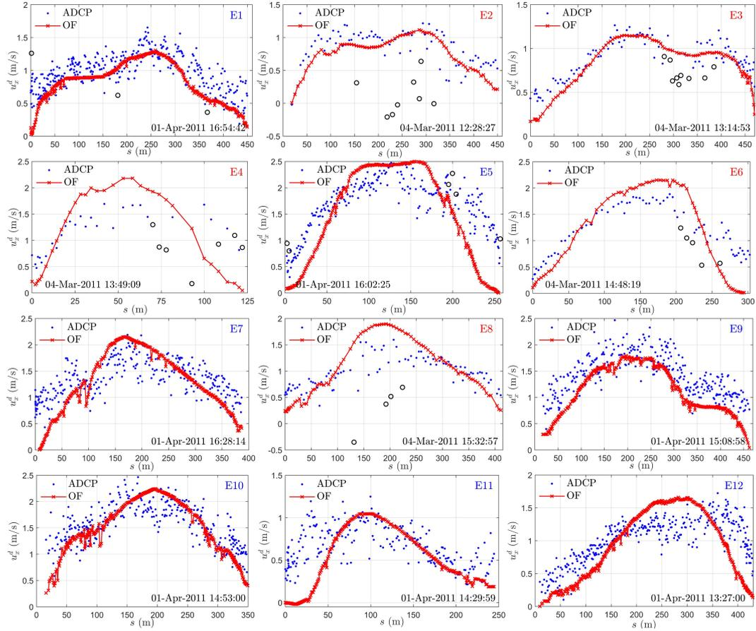
**Figure A5.** A comparison of depth-averaged velocity component along  $x$  from ADCP surveys and CFD modeling at E1 - E12. Black circles denote measured outliers visually determined from Figure A5 or A6.
