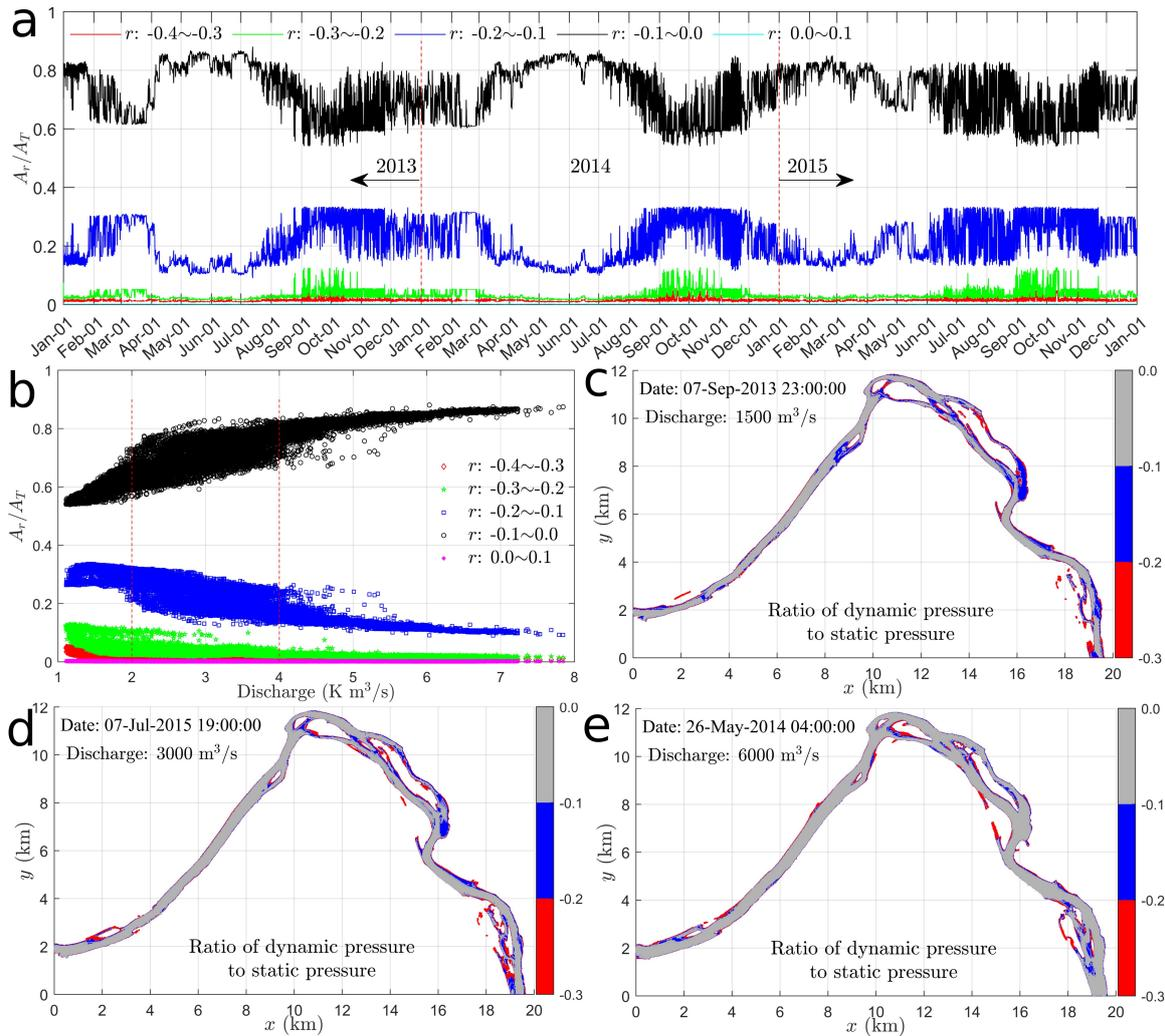
**Figure 11.** The variations of the relative pressure ratio area ( $A_r/A_T$ ) with time (a) and discharge (b), as well as the spatial distribution of each pressure ratio range at low (c), medium (d), and high (e) flow conditions.
