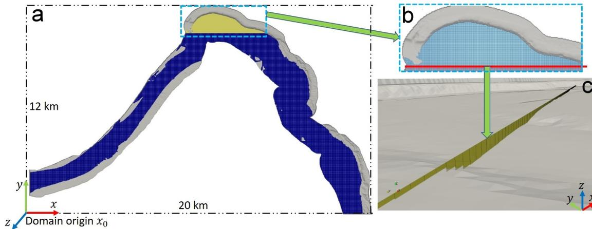
**Figure 2.** Horizontal and vertical computational meshes. (a) Top view showing the horizontal mesh over the whole domain. (b) Top view showing the details of horizontal mesh near LI. (c) 3D view showing details of the vertical mesh structure.
