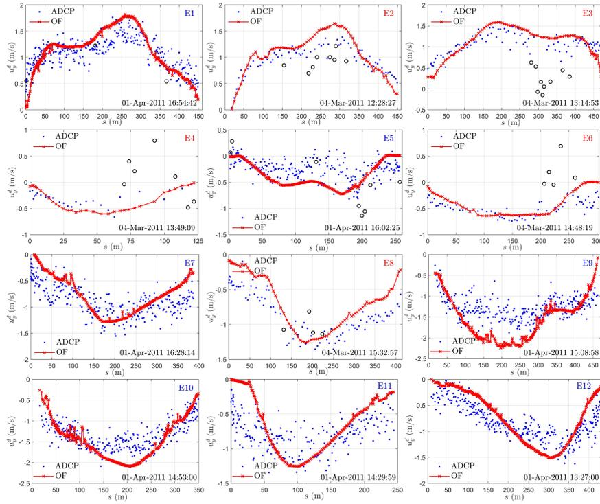
**Figure A6.** A comparison of depth-averaged velocity component along  $y$  from ADCP surveys and CFD modeling at E1 - E12. Black circles denote measured outliers visually determined from Figure A5 or A6.
