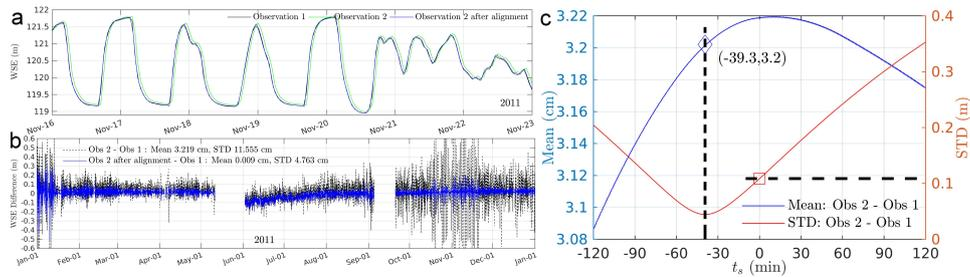
**Figure A7.** A comparison of WSE at 100B from observation 1, observation 2, and observation 2 after alignment (a), the differences in WSE between observation 1 and observation 2 and that between observation 1 and observation 2 after alignment (b), and the mean and standard deviation between observation 1 and observation 2 with a time shift  $t_s$  (c).
