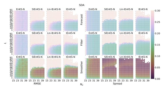
Figure 7. Lag length L vertical axis, ensemble size  $N_e$  horizontal axis. SDA, adaptive inflation, shift S=1, linear observations,  $\Delta t=0.05$ .
