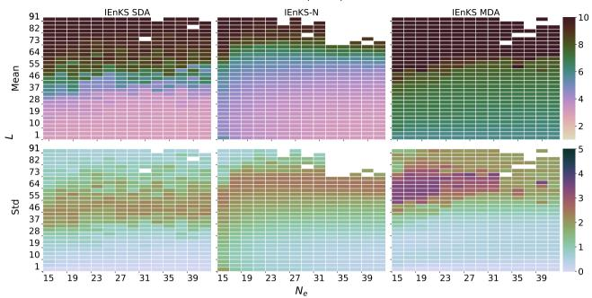
Figure 13. Iterations per cycle versus lag L in the vertical axis and ensemble size  $N_e$  in the horizontal axis. Mean (top panel) and standard deviation (bottom panel) of iterations used per cycle from simulations generating Figs. 5, 7 and 9 are presented.
