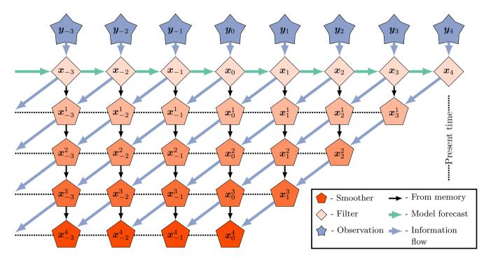
**Figure 2.** Lag= 4, shift= 1 EnKS. Observations are assimilated sequentially via the filter cost function and a retrospective re-analysis is applied to all ensemble states within the lag window stored in memory. Adapted from Asch et al. (2016).
