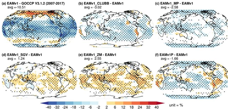
**Figure 5.** Total cloud fraction between (a) EAMv1 and the version 3.1.2 of the GOCCP total cloud fraction (Chepfer et al., 2010) averaged over 2007-2017; (b) EAMv1\_CLUBB and EAMv1; (c) EAMv1\_MP and EAMv1; (d) EAMv1\_SGV and EAMv1; (e) EAMv1\_ZM and EAMv1; and (f) EAMv1P and EAMv1. Model cloud fractions are derived from the CALIPSO cloud simulator (Chepfer et al., 2008) sampled at 1:30 PM local time.
