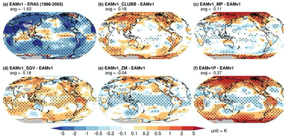
655 **Figure 6.** Estimated inversion strength (EIS; unit = K). The EIS computed from European Centre for Medium-Range Weather Forecasts' (ECMWF's) fifth generation global meteorological reanalysis (ERA5) (Hersbach et al., 2019) is used for the comparison with EAMv1.
