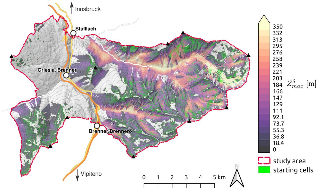
**Figure 8.** Flow-Py simulation results of snow avalanche runout and intensity ( $Z_{max}^{\delta}$ ) in complex terrain on a regional scale. The simulation took 3 h and 45 min. The map utilizes data from ©OpenStreetMap contributors 2021. Distributed under the Open Data Commons Open Database License (ODbL) v1.0. and Land Tirol (data.tirol.gv.at) issued under a Creative Commons Attribution 4.0 International (CC BY 4.0) license.
