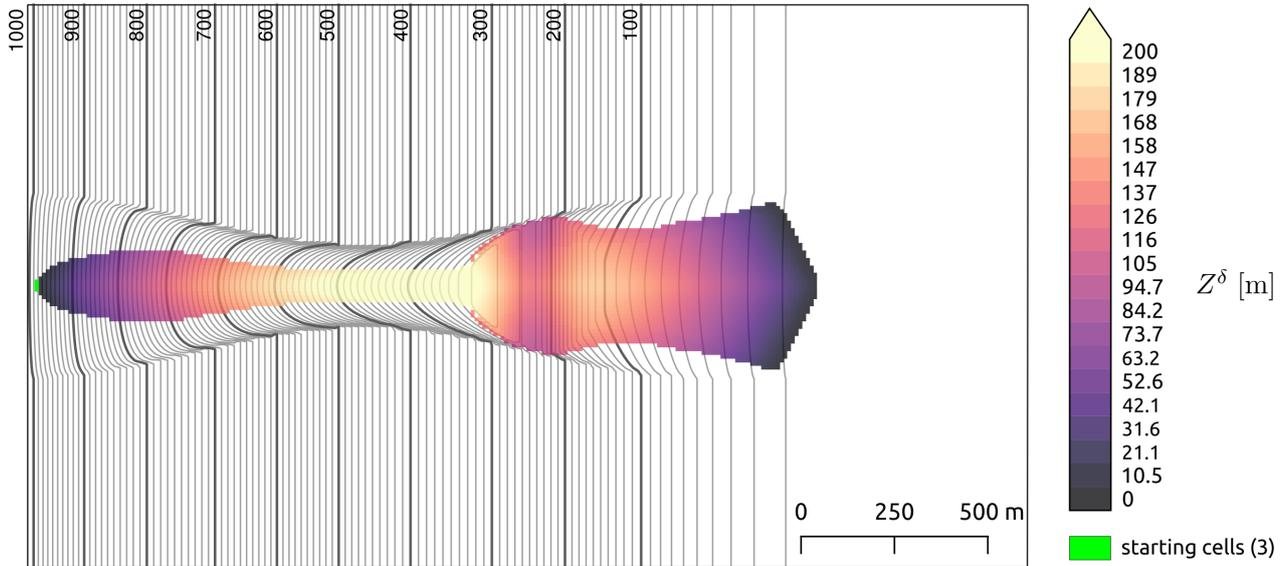
**Figure 5.** GMF runout modeled with Flow-Py on a parabolic slope with a channel and a dam that crosses the terrain at 1350 m with  $\alpha = 25^\circ$ ,  $exp = 8$ ,  $R_{stop} = 3 \cdot 10^{-4}$  and  $Z_{lim}^\delta = 8,849m$ . The colors show the value of  $Z_{max}^\delta$  which is associated to maximum kinetic energy. The topography is a simple parabolic slope connected to a flat plane.
