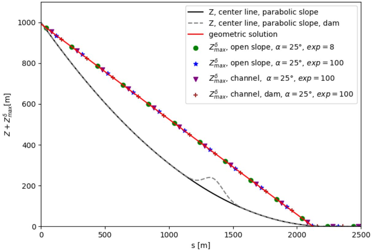
**Figure 6.** Geometric solution for the stopping criteria (red line) represented by the  $\alpha$ -line from starting to the runout points with  $Z_{max}^{\delta}$  values for the center lines of scenarios presented in Sect. 3.1 and 3.2 (black line), and 3.3 (black dashed line).
