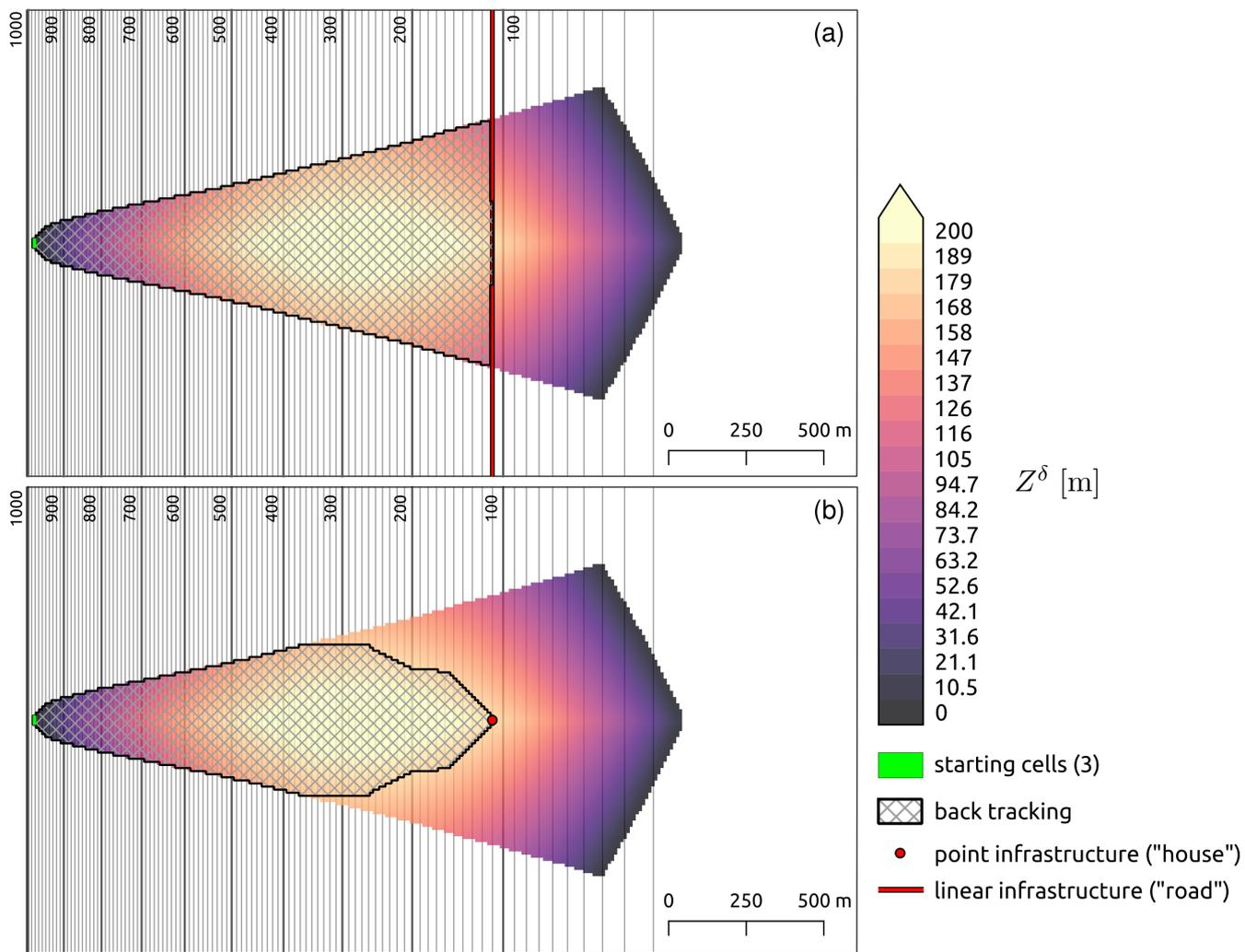
**Figure 9.** GMF runout modeled with Flow-Py and results of the back-tracking extension with  $\alpha = 25^\circ$ ,  $exp = 8$ ,  $R_{stop} = 3 \cdot 10^{-4}$  and  $Z_{lim}^\delta = 8,849m$ . The textured areas highlight starting, transit or runout zones associated with endangering linear infrastructure (a) or a building (b). The topography is a simple parabolic slope connected to a flat plane.
