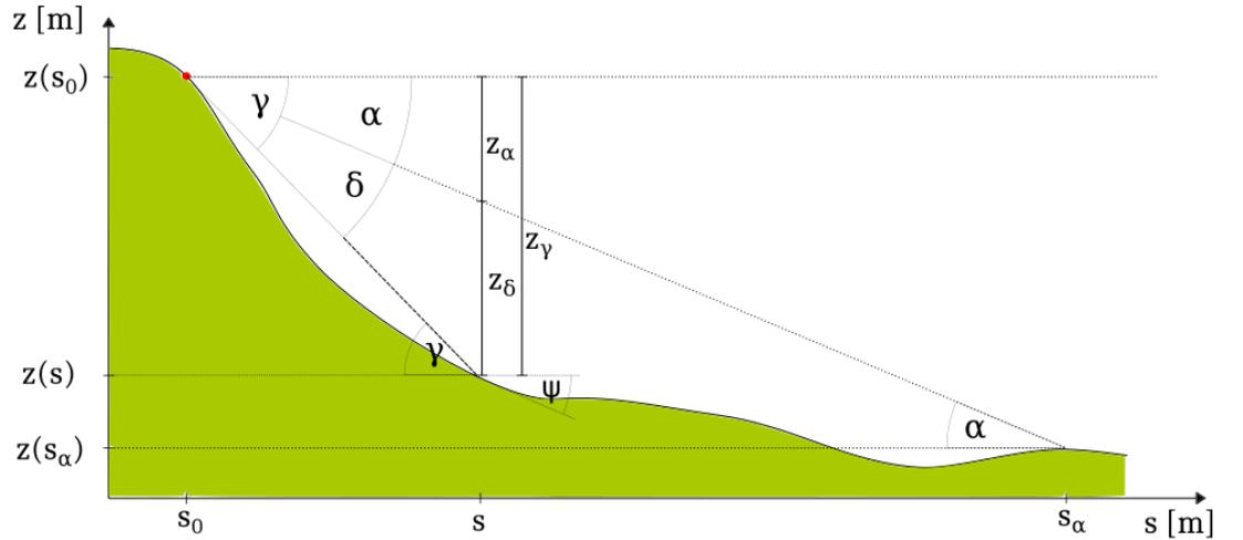
**Figure 1.** GMF path with altitude  $z(s)$ , projected travel distance  $s$  and local slope angle  $\psi$  with starting point  $s_0, z(s_0)$  and runout point  $s_\alpha, z(s_\alpha)$ . The corresponding geometric quantities are directly related to the runout angle  $\alpha$  concept and include the local travel angle  $\gamma$ , with corresponding total altitude change  $z_\gamma$  and the process intensity measure  $z_\delta$  with angle  $\delta$ .
