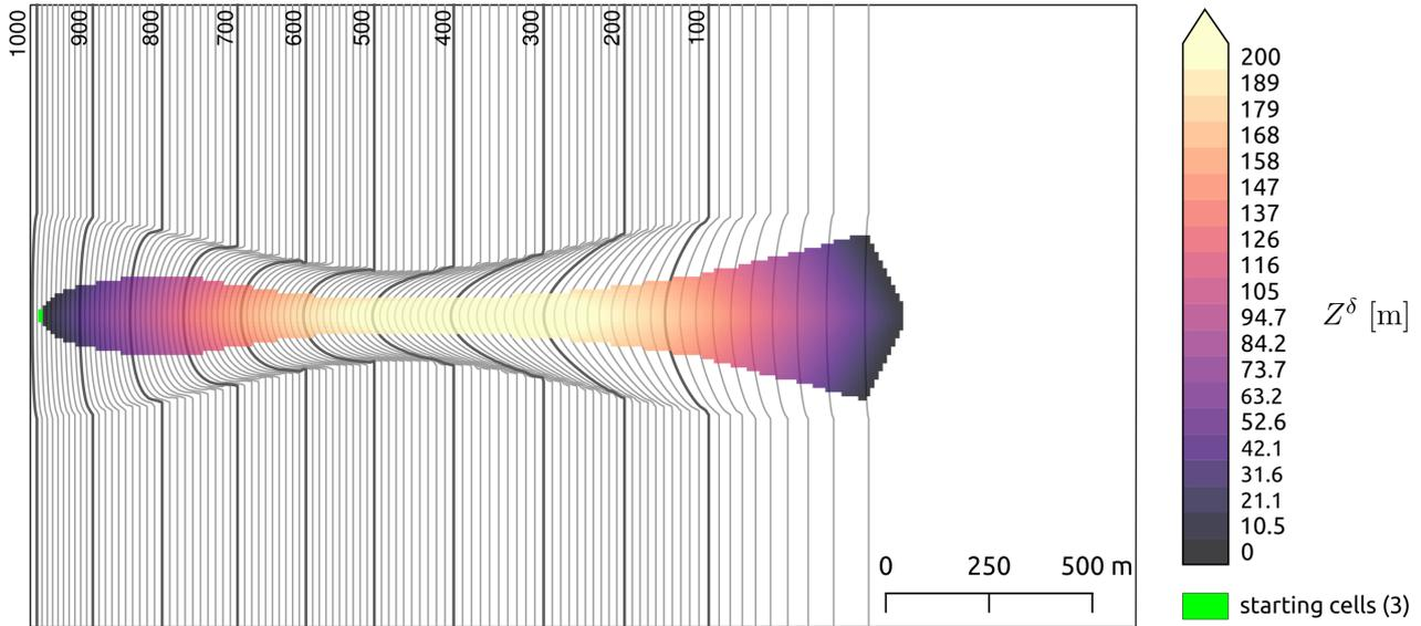
**Figure 4.** GMF runout modeled with Flow-Py on a parabolic slope with a channel with  $\alpha = 25^\circ$ ,  $exp = 8$ ,  $R_{stop} = 3 \cdot 10^{-4}$  and  $Z_{lim}^\delta = 8,849m$ . The colors show the value of  $Z_{max}^\delta$ , which is associated to maximum kinetic energy. The topography is a simple parabolic slope connected to a flat plane.
