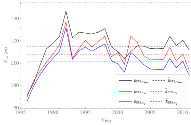
570 Figure 8. Values of limit (saturated) values E_{EFS, \infty_w} of the extended power law \lambda_w(E) (red), E_{EFS, \infty_q} of the extended quadratic model \lambda_q(E) (blue), and theoretical value E_{EFS, \infty_{\text{teor}}} determined by Bednar et al. (2020) approximated from annual averages of the error growth rate \lambda_{EFS}(E) of the ECMWF forecasting system's 500 hPa geopotential height values (Northern Hemisphere (20°–90°)) calculated as differences between two operational forecasts issued with one day lag but valid on the same day. The average value of \bar{E}_{EFS, \infty_w} = 114 \pm 7 m (red, dashed), \bar{E}_{EFS, \infty_q} = 111 \pm 7 m (blue, dashed), and \bar{E}_{EFS, \infty_{\text{teor}}} = 118 \pm 7 m (black, dashed).
