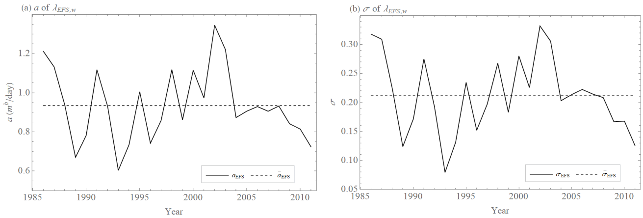
560 Figure 6. Values of coefficients a (a) and exponents \sigma (b) of the extended power law \lambda_w(E) (Eq. (26)) approximated from annual averages of the error growth rate \lambda_{EFS}(E) of the ECMWF forecasting system's 500 hPa geopotential height values (Northern Hemisphere ( 20^\circ – 90^\circ )) calculated as differences between two operational forecasts issued with one day lag but valid on the same day (black) and the average value of coefficients \bar{a}_{EFS} = 0.93 \pm 0.18 m \sigma /day and exponents \bar{\sigma}_{EFS} = 0.21 \pm 0.07 over all years (black, dashed).
