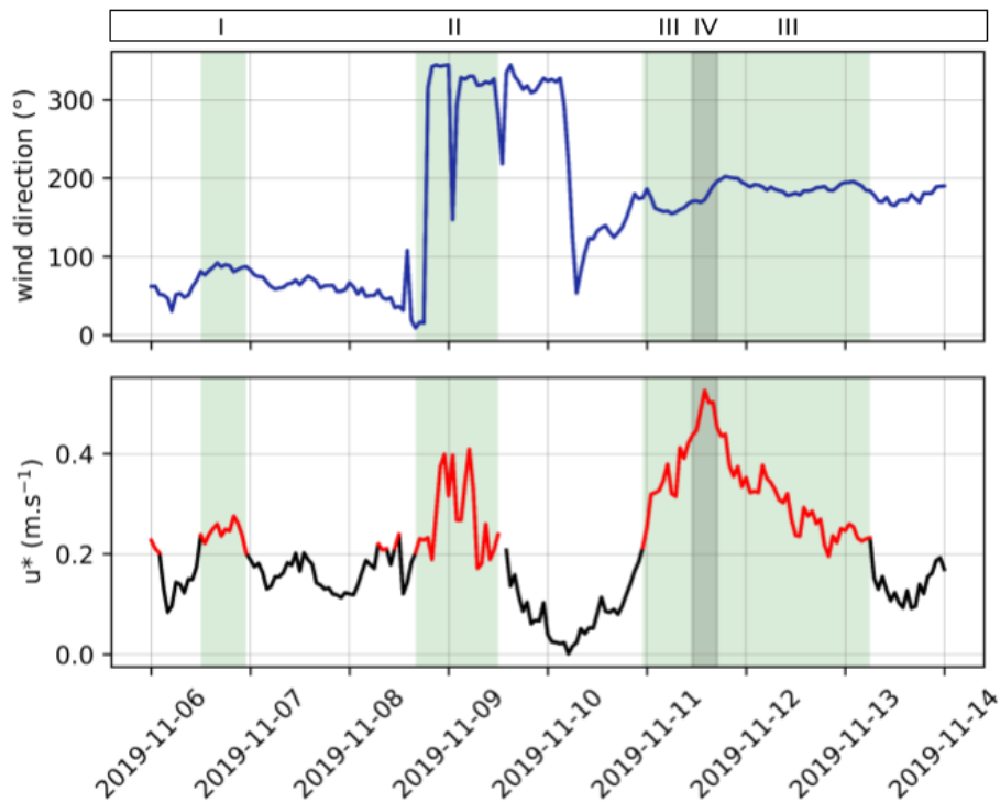
Figure 3. Time series for wind direction (top) and surface friction velocity at 2m (bottom) measured in the period between the successive TLS measurements. The values displayed are an average of measurements taken at 2 m, 6 m and 10 m height. The green-colored areas (I to III) correspond to the time periods for which snow movement was assumed to occur. The darker area (IV) shows the time span during which precipitation was measured by the radar. Source: Cox et al. (2021).
