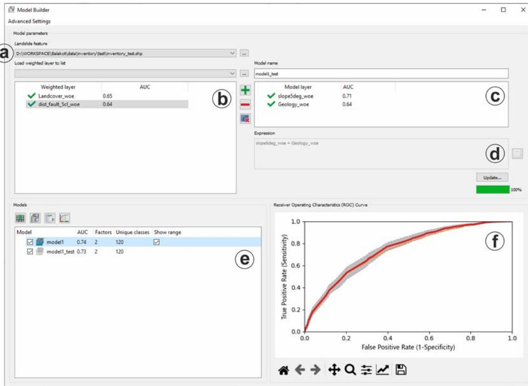
**Figure 3: Model Builder GUI with its integral parts: a – Landslide inventory collection; b – weighted layer collection; c – model layer collection; d – model generating expression; e – models collection; f – ROC curves.**
