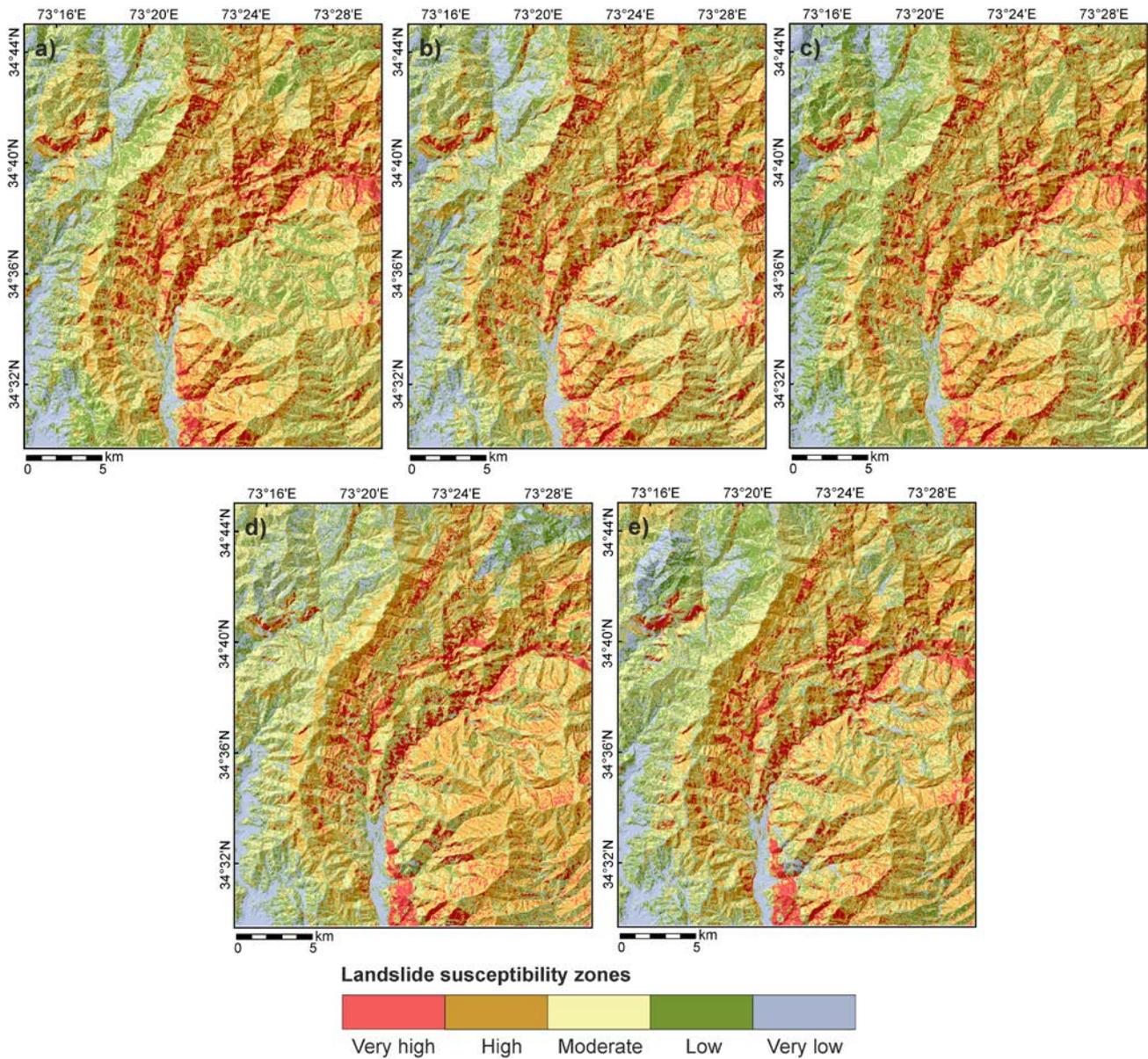
470 **Figure 12** Landslide susceptibility zones based on different models: a) WoE; b) LR\_d; c) LR\_c; d) ANN\_d; e) ANN\_c. *Very high* contains about 50%, *High* about 30%, *Moderate* about 15%, *Low* about 4% and *Very low* about 1% of all landslide pixels.
