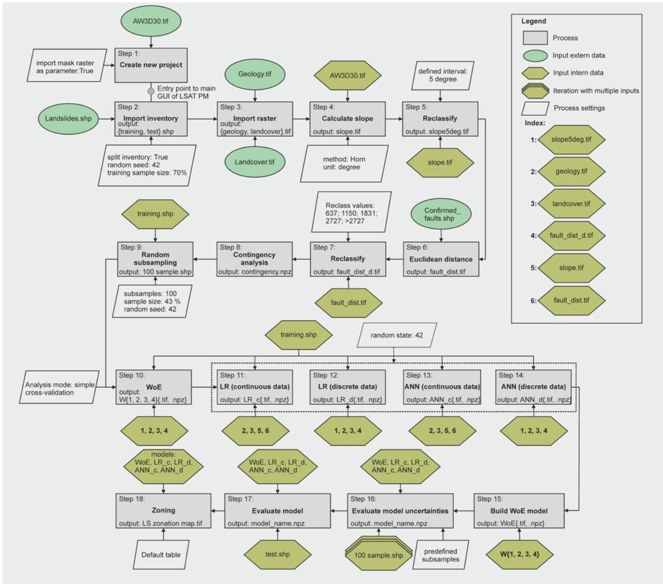
Figure 6: Workflow applied to the test dataset.
