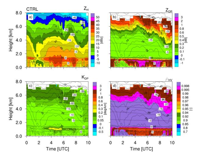
**Figure 5.** Synthetic QVPs of horizontal reflectivity  $Z_{\rm H}$ , differential reflectivity  $Z_{\rm DR}$ , specific differential phase  $K_{\rm DP}$ , and cross-correlation coefficient  $\rho_{\rm hv}$  for the CTRL run and applying the B-PRO<sub>def</sub> setup. Radar variable color scales are identical to the ones applied in Fig. 1. Also shown are contours of air temperature.
