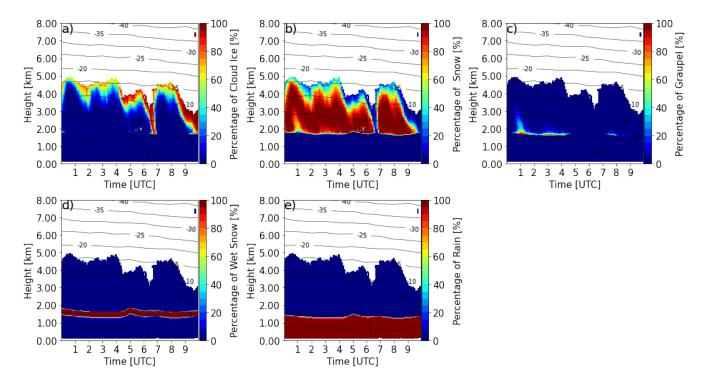
**Figure 7.** Time series of hydrometeor percentage retrieved from the observed QVPs with HCA-Pejcic for cloud ice (a), snow (b), graupel (c), wet snow (d) and rain (e).
