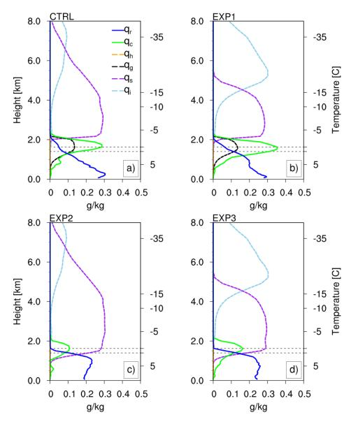
Figure 9. Half-hourly averaged QVPs of modeled hydrometeor mixing ratio around 04:00UTC on 16 Nov 2014. On the right axis, air temperatures corresponding to the heights are denoted. Dashed gray lines indicate temperature thresholds of  $\pm 0.5^{\circ}$ C in the melting layer.
