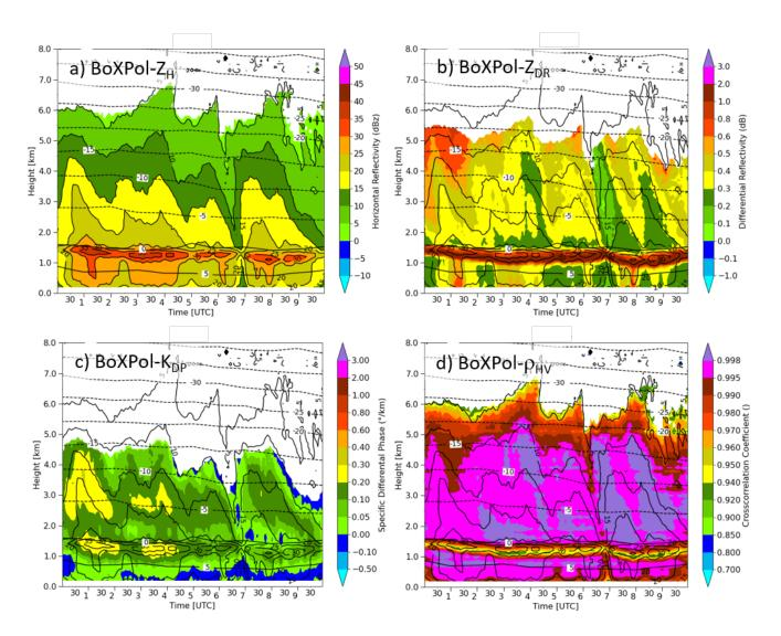
**Figure 1.** Time series of quasi-vertical profiles measured with the polarimetric X-band radar in Bonn (BoXPol) on 16 Nov 2014. Panels show (a) horizontal reflectivity  $Z_{\rm H}$ , (b) differential reflectivity  $Z_{\rm DR}$ , (c) specific differential phase  $K_{\rm DP}$ , and (d) cross-correlation coefficient  $\rho_{\rm hv}$ . Overlaid solid black contours depict the  $Z_{\rm H}$  field in 5-dBZ increments, while black dashed lines indicate the COSMO isotherms for the radar location.
