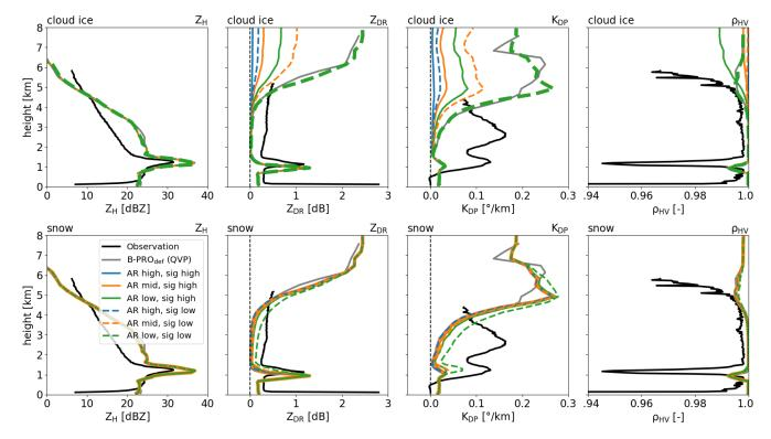
Figure 12. As Fig. 11, but for model experiment EXP3. No graupel panel is shown here, since graupel mixing ratios in this experiment are too low to produce noticeable contributions to the radar signal.
