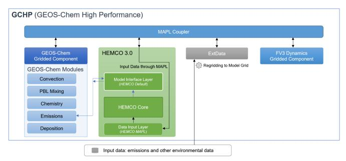
**Figure 5. HEMCO 3.0 implementation in the GEOS-Chem high performance model (GCHP).** GCHP operates under the MAPL coupling framework in a MPI parallel environment. The ExtData component reads all data into MAPL, re-gridding them to the model grid, and the input data are retrieved by the HEMCO MAPL implementation of the Data Input Layer. After emissions are processed by the HEMCO Core, they are exported to GEOS-Chem through the HEMCO default Model Interface Layer.
