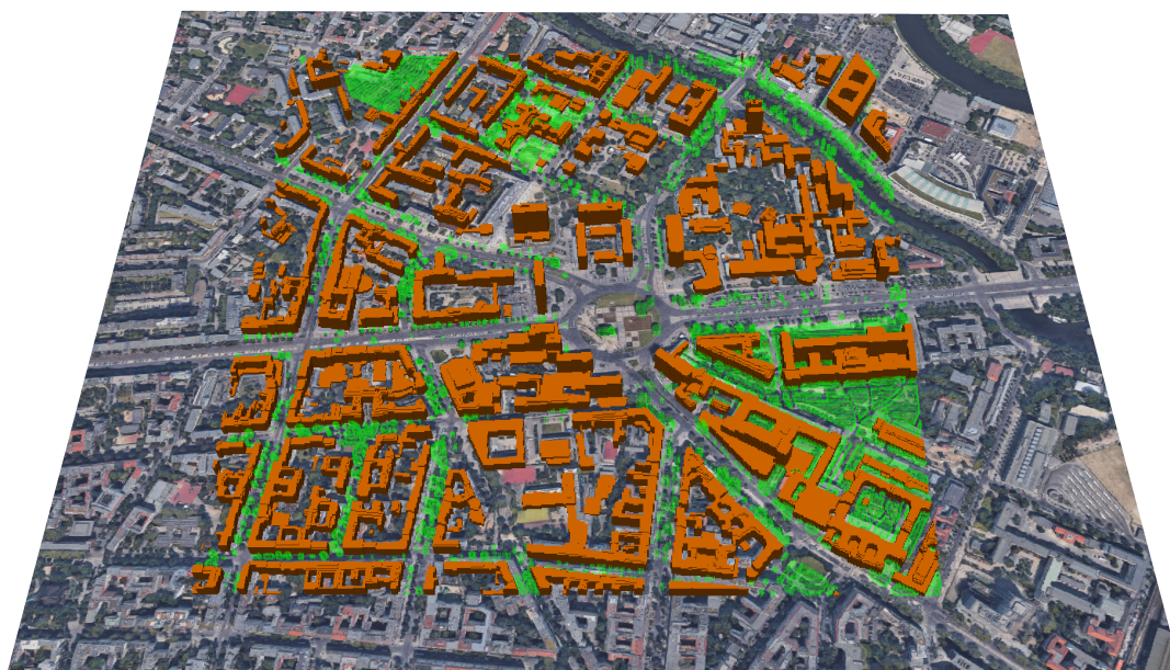
Figure 2. An aerial view of the realistic urban configuration showing the 3-D buildings (fitted to the grid) and the plant canopy boxes (trees, shown in green points). The configuration is centred around Ernst-Reuter-Platz in Charlottenburg in Berlin (N52° 30.8' E48° 19.31'). The copyright for the underlying satellite image is held by GeoBasis-DE/BKG (©2009), Google
