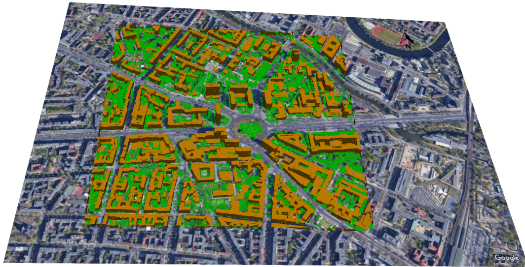
Figure 2. An aerial view of the realistic urban configuration showing the 3-D buildings (fitted to the grid) and the plant canopy boxes (trees, shown in green points). The configuration is centred around Ernst-Reuter-Platz in Charlottenburg in Berlin ( N52^{\circ}30.8' E48^{\circ}19.31' ). The copyright for the underlying satellite image is held by GeoBasis-DE/BKG (©2009), Google
