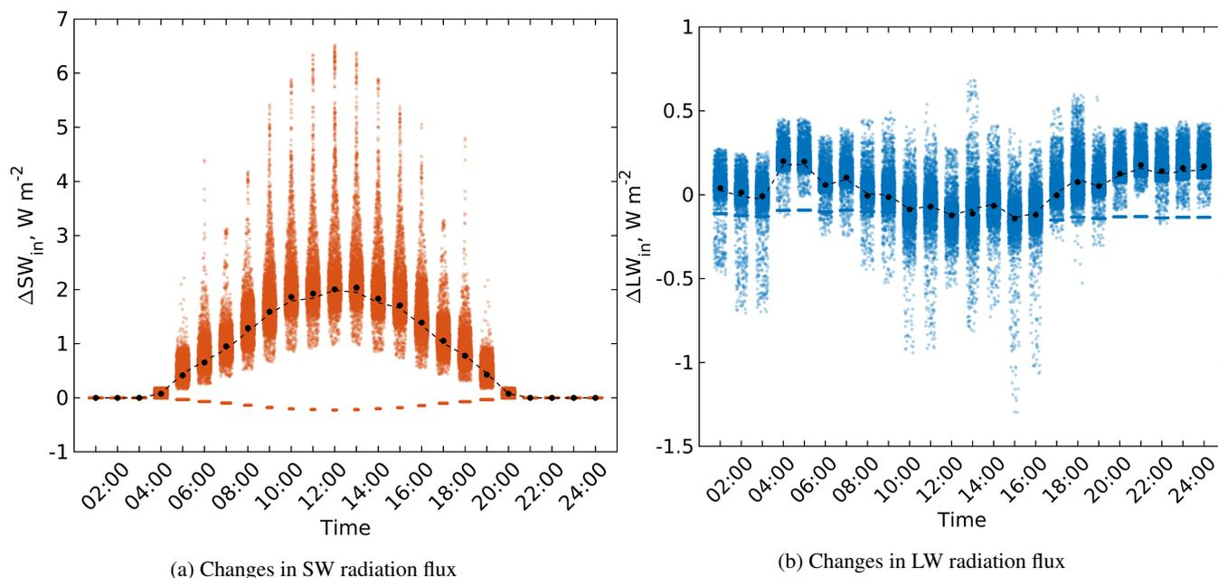
**Figure 17.** Changes in the received SW and LW irradiance within the focus domain of the simple urban configuration when considering multiple reflections (RTM\_08) compared to RTM\_07. Violin, mean, and median colours are used in the same way as in Fig. 4
