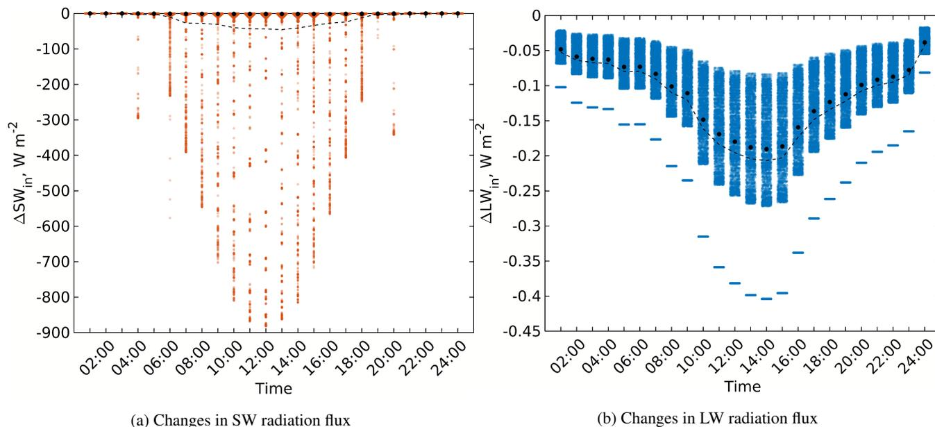
**Figure 7.** Changes in the received SW and LW irradiance within the focus domain of the simple urban configuration when considering vegetation interaction with SW solar radiation (RTM\_03) compared to the RTM\_02. Violin, mean, and median colours are used in the same way as in Fig. 4
