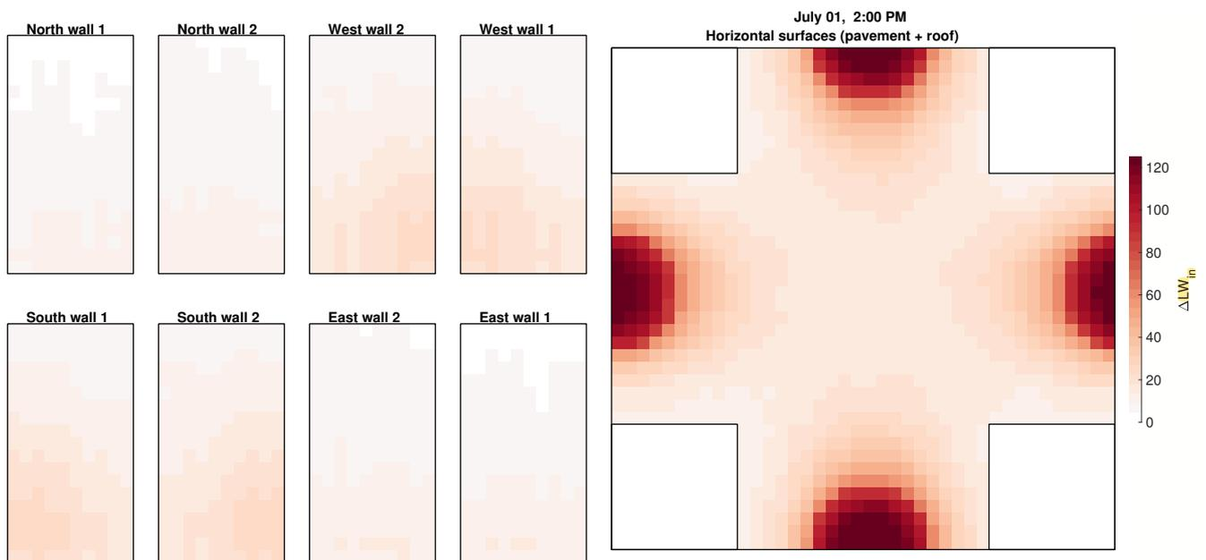
**Figure 12.** Changes in the received LW radiation flux within the focus domain of the simple urban configuration when including vegetation interaction with LW radiation (RTM\_05) compared to RTM\_04. Walls, roofs, and pavements are folded the same as as in Fig. 6.
