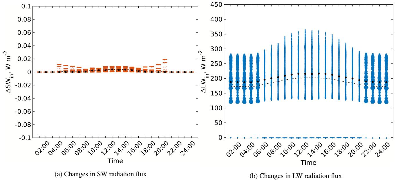
**Figure 9.** Changes in the received SW and LW irradiance within the focus domain of the simple urban configuration when considering surface thermal emissions (RTM\_04) compared to the RTM\_03. Violin, mean, and median colours are used in the same way as in Fig. 4
