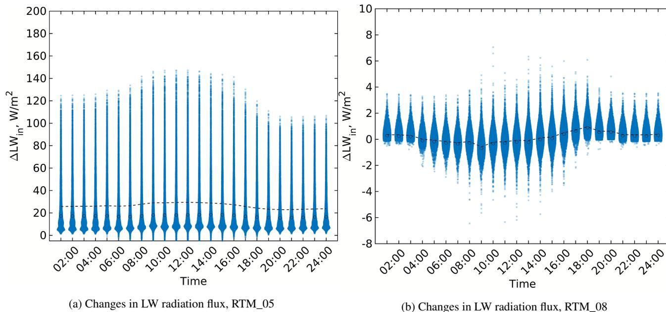
**Figure 22.** Changes in the received LW irradiance for the surfaces of the realistic urban configuration when considering (a) the vegetation interaction with LW radiation (RTM\_05) and (b) the multiple reflections (RTM\_08). Violin, mean, and median colours are used in the same way as in Fig. 4
