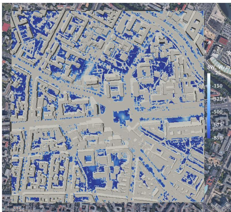
**Figure 21.** Changes in the received SW radiation flux for the realistic urban configuration at 10:00 solar time due to including the vegetation interaction with the SW radiative transfer (RTM\_03). The copyright for the underlying satellite image is held by GeoBasis-DE/BKG (©2009), Google
