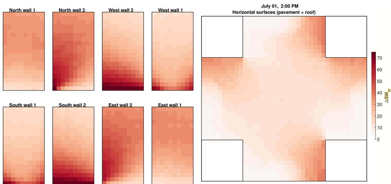
**Figure 14.** Changes in the received SW radiation flux within the focus domain of the simple urban configuration when considering one reflection (RTM\_06) compared to RTM\_05. Walls, roofs, and pavements are folded the same way as in Fig. 6.
