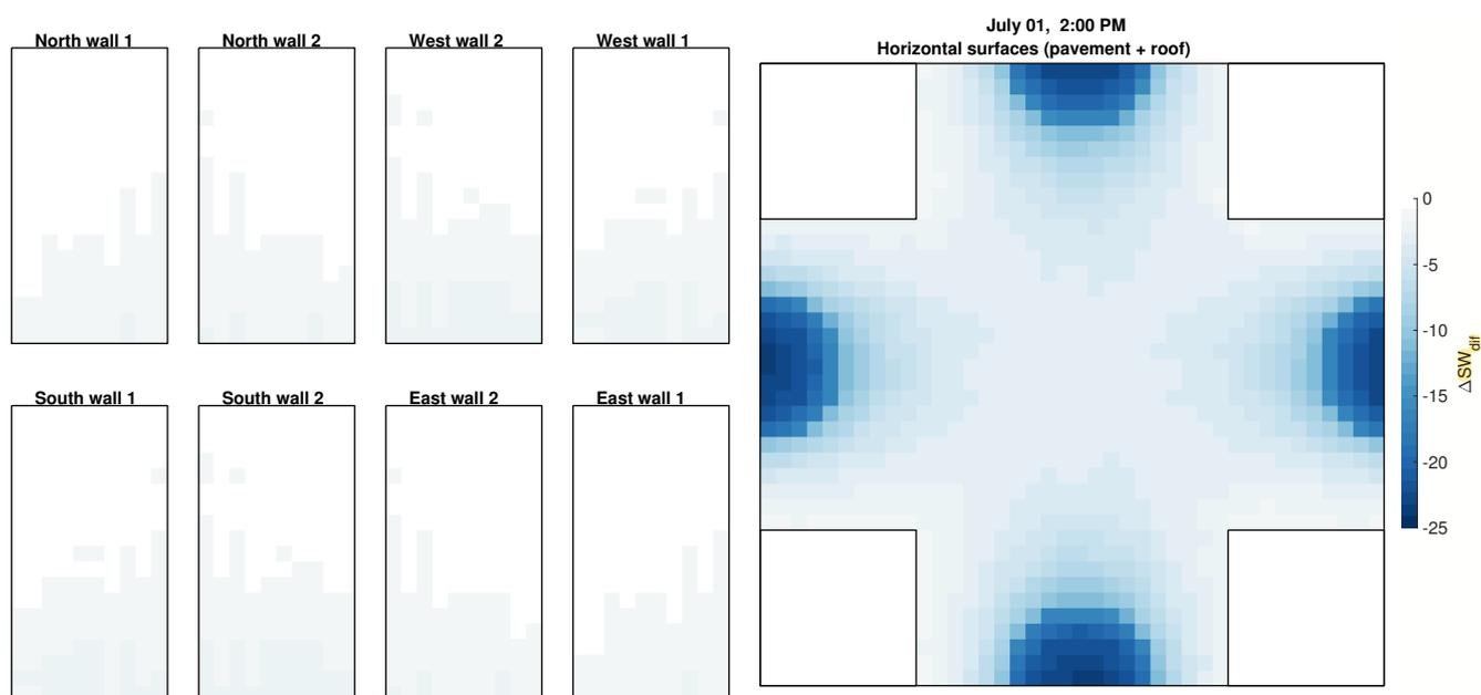
**Figure 8.** Changes in the received diffuse SW radiation flux within the focus domain of the simple urban configuration when considering vegetation interaction with SW solar radiation (RTM\_03) compared to the RTM\_02. Walls, roofs, and pavements are folded the same as in Fig. 6
