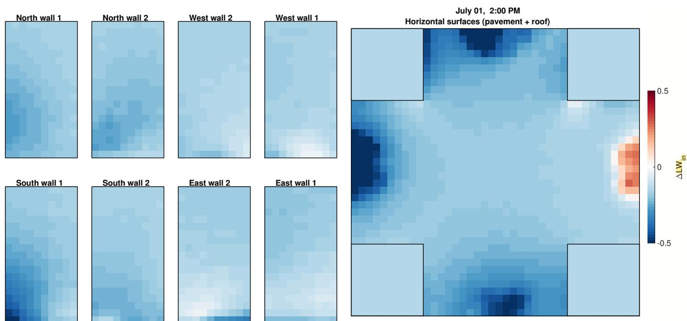
**Figure 16.** Changes in the received LW radiation flux within the focus domain of the simple urban configuration when considering vegetation interaction with the reflected radiation (RTM\_07) compared to RTM\_06. Walls, roofs, and pavements are folded the same as as in Fig. 6.
