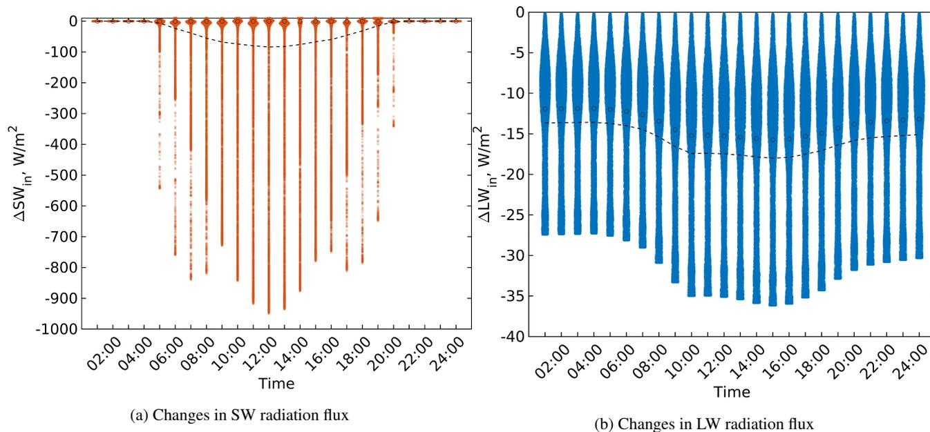
**Figure 20.** Changes in the received SW and LW irradiance for the surfaces of the realistic urban configuration when considering vegetation interaction with SW solar radiation (RTM\_03). Violin, mean, and median colours are used in the same way as in Fig. 4
