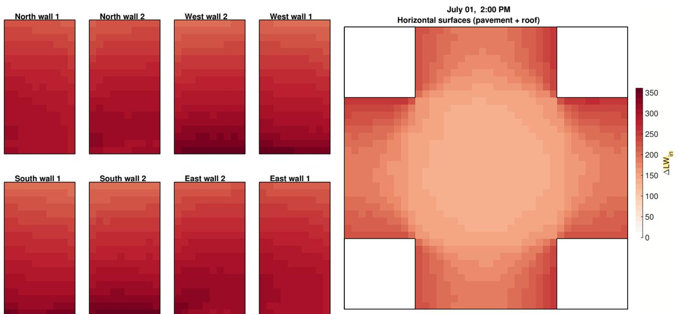
**Figure 10.** Changes in the received diffuse LW radiation flux within the focus domain of the simple urban configuration when considering surface thermal emissions (RTM\_04) compared to the RTM\_03. Walls, roofs, and pavements are folded the same as in Fig. 6.
