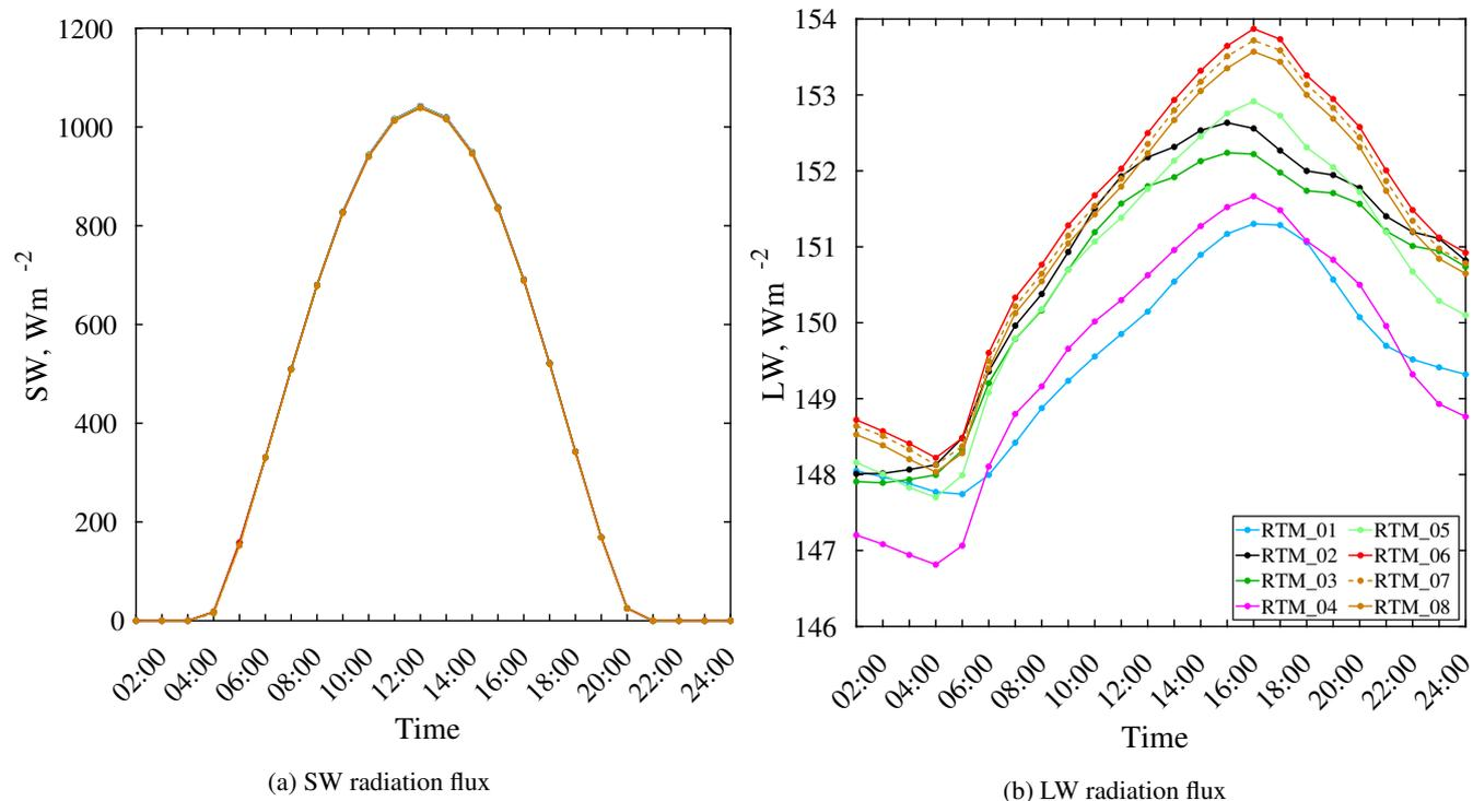
**Figure 3.** The daily course of (a) incoming shortwave and (b) incoming longwave radiation fluxes for the top of urban layer of the simple urban configuration at  $52^{\circ}\text{N}$  on July 1st for different RTM configurations
