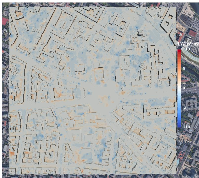
**Figure 23.** Changes in the received LW radiation flux for the realistic urban configuration at 12:00 solar time due to including multiple reflections (RTM\_08). The copyright for the underlying satellite image is held by GeoBasis-DE/BKG (©2009), Google
