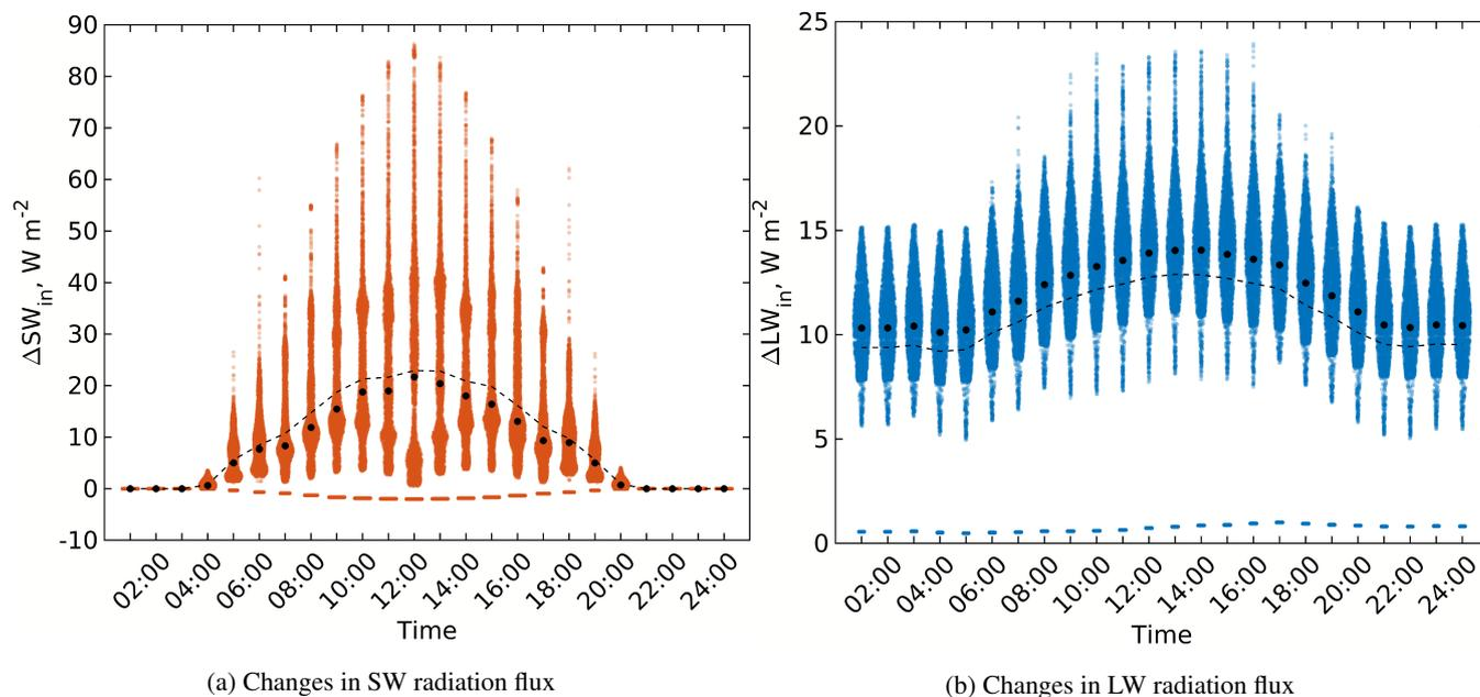
**Figure 13.** Changes in the received SW and LW irradiance within the focus domain of the simple urban configuration when considering one reflection (RTM\_06) compared to RTM\_05. Violin, mean, and median colours are used in the same way as in Fig. 4
