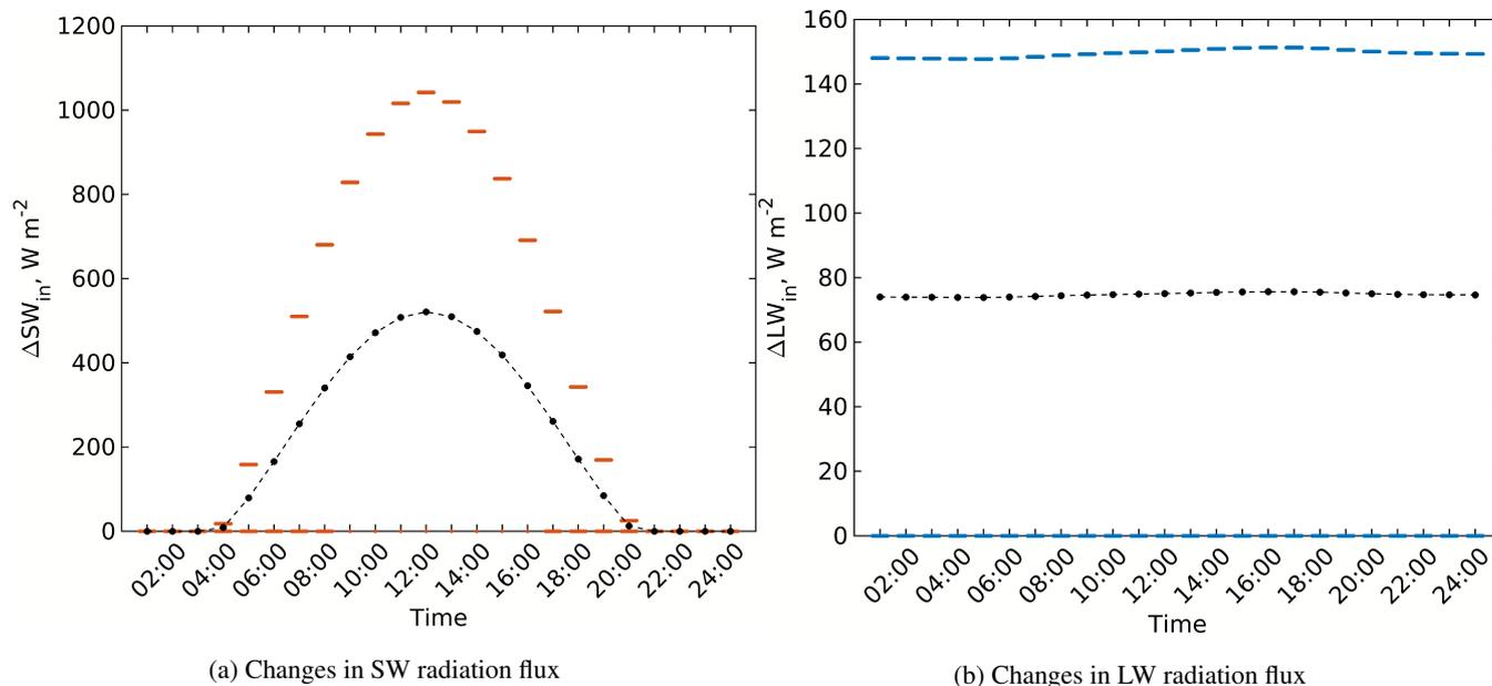
**Figure 4.** Changes in the received SW and LW irradiance within the focus domain of the simple urban configuration when applying the simple RTM (RTM\_01) compared to the neutral case (RTM\_00). The colour of the SW irradiance violin plots is orange and those of the LW irradiance is blue. The mean values are shown in black dashed line and the median values are shown in black circles
