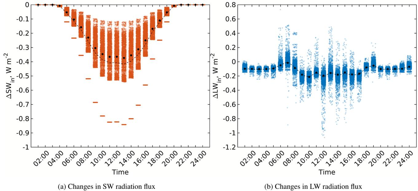
**Figure 15.** Changes in the received SW and LW irradiance within the focus domain of the simple urban configuration when considering vegetation interaction with the reflected irradiance (RTM\_07) compared to RTM\_06. Violin, mean, and median colours are used in the same way as in Fig. 4
