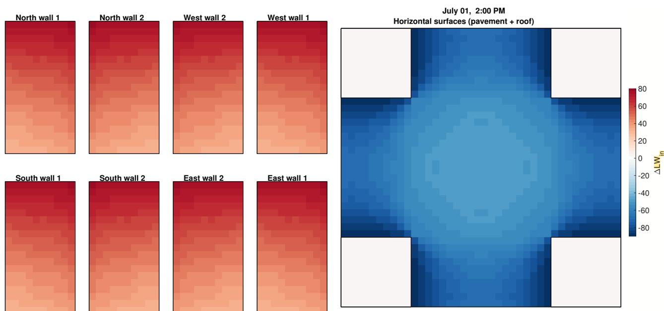
**Figure 6.** Changes in the received LW radiation flux within the focus domain of the simple urban configuration when considering the surface sky view factors (RTM\_02) compared to the RTM\_01. Walls (left plot), roofs (in the centre of the right plot), and pavements (rectangles on all four sides in the right plot) are folded. See the details of the focus domain of the simple urban configuration in Fig. 1
