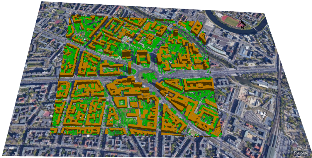
Figure 2. An aerial view of the realistic urban configuration showing the 3-D buildings (fitted to the grid) and the plant canopy boxes (trees, shown in green points). The configuration is centred around Ernst-Reuter-Platz in Charlottenburg in Berlin ( N52^{\circ}30.8' E48^{\circ}19.31' ). The copyright for the underlying satellite image is held by GeoBasis-DE/BKG (©2009), Google
