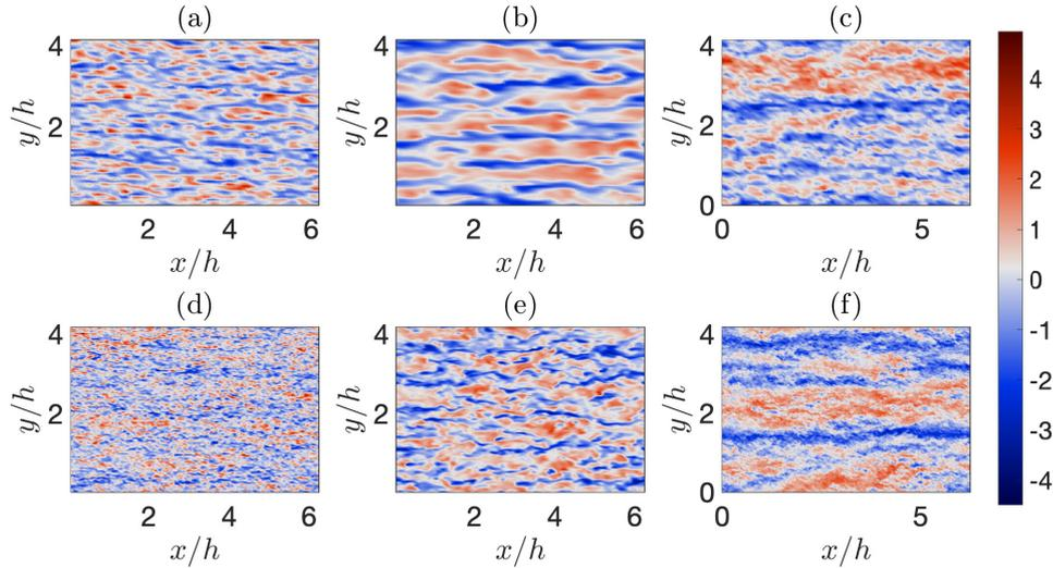
**Figure 6.** Instantaneous snapshots of normalized streamwise velocity fluctuations at  $z/h \approx 0.1$  from the simulations FV64 (a), FV64\* (b), PSFD64 (c), FV160 (d), FV160\* (e) and PSFD160 (f). The normalized velocity fluctuation is defined as  $(u - \langle u \rangle_{xy})/u''$ , where averages (and fluctuations therefrom) are evaluated in space over the selected horizontal plane.
