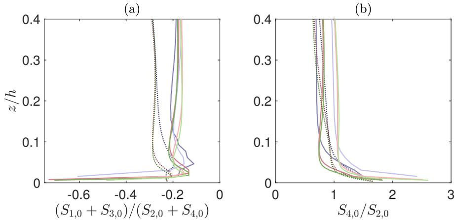
**Figure 8.** Vertical structure of event ratios: (a) ratio of negative to positive contributions to the momentum flux; (b) ratio of sweeps to ejections. Lines and symbols are defined as in Table 1 Fig. 1.
