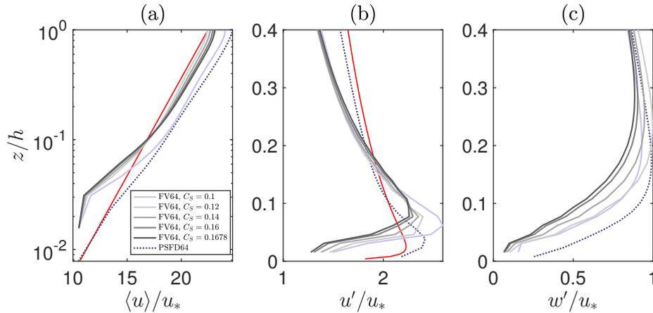
**Figure A1.** Vertical structure of streamwise velocity (a), streamwise velocity RMS (b), vertical velocity RMS (c). Red lines denote the phenomenological logarithmic-layer profile (a) and the analytical expressions from similarity theory (Stull, 1988) (b, dark to light gray,  $C_S = 0.1$  to  $C_S = 0.1678$ ; full circles, PSFDc).
