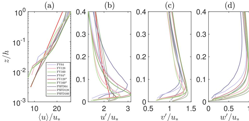
**Figure 1.** Vertical structure of mean streamwise velocity  $\langle u \rangle / u_*$  (a), streamwise velocity RMS (b), cross-stream velocity RMS (c) and vertical velocity RMS (d). The red line in (a) denotes the reference logarithmic profile and the red line in (b) is a reference profile from Hultmark et al. (2013).
