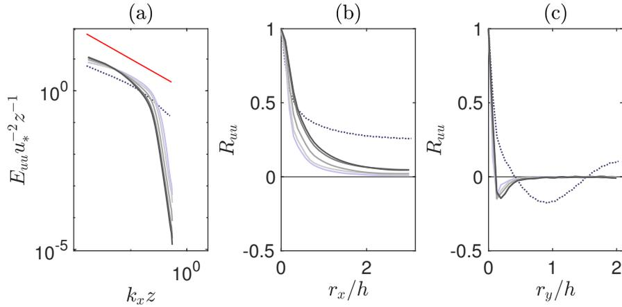
**Figure A2.** Vertical-structure Normalized one-dimensional spectrum of streamwise velocity at height  $z/h \approx 0.1$  (a); one-dimensional spatial autocorrelation of streamwise velocity RMS at height  $z/h \approx 0.1$  along the streamwise direction (b); vertical-velocity RMS and along the cross-stream direction (c). Circles Lines as in Fig. A1. Red line, linear interpolation scheme; x-marks, QUICK interpolation scheme; full circles, PSFD  $(k_x z)^{-1}$ .
