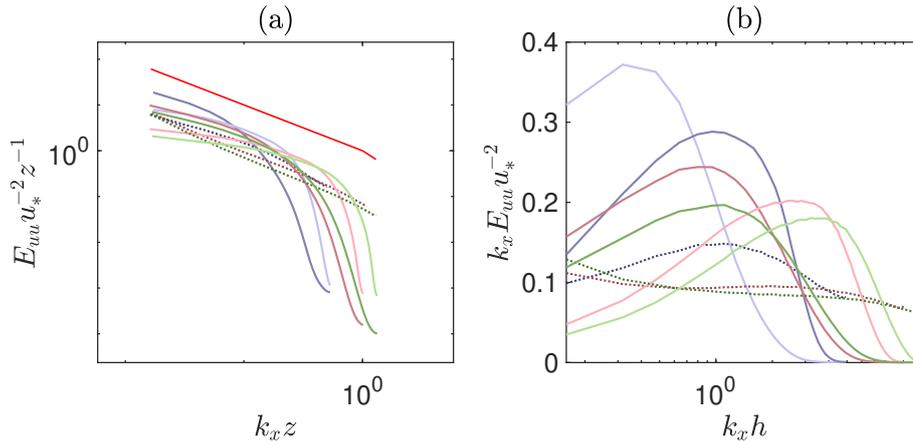
**Figure 3.** (a) Normalized one-dimensional spectrum of streamwise velocity at height  $z/h \approx 0.1$ . Solid red line,  $(k_x z)^{-1}$  in the production range and  $(k_x z)^{-5/3}$  in the inertial sub-range. All the other lines as in Fig. 1. (b) Premultiplied one-dimensional spectrum of streamwise velocity at  $z/h \approx 0.1$ .
