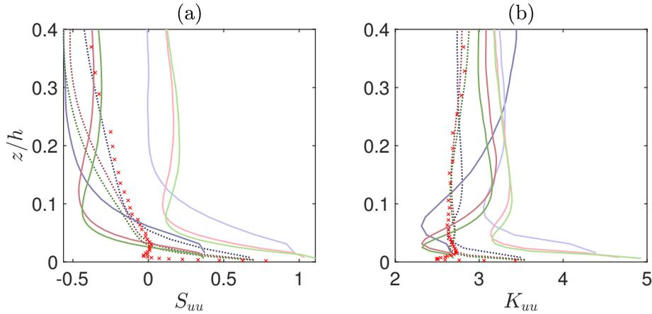
**Figure 2.** Vertical structure of skewness of streamwise velocity (a) and kurtosis of streamwise velocity (b) and transfer efficiency coefficient (c). Lines and symbols are defined in Table 1 Fig. 1. The red x-marks denote the measurements from Monty et al. (2009), digitalized by the authors.
