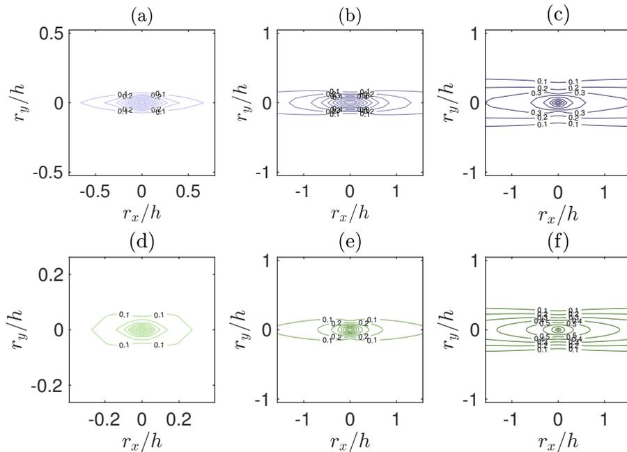
**Figure 4.** Contours of two-dimensional spatial autocorrelation of streamwise velocity at height  $z/h \approx 0.1$ , from the simulations FV64 (a), FV64\* (b), PSFD64 (c), FV160 (d), FV160\* (e) and PSFD160 (f). Contour levels from 0.1 to 0.9 with increments of 0.1.
