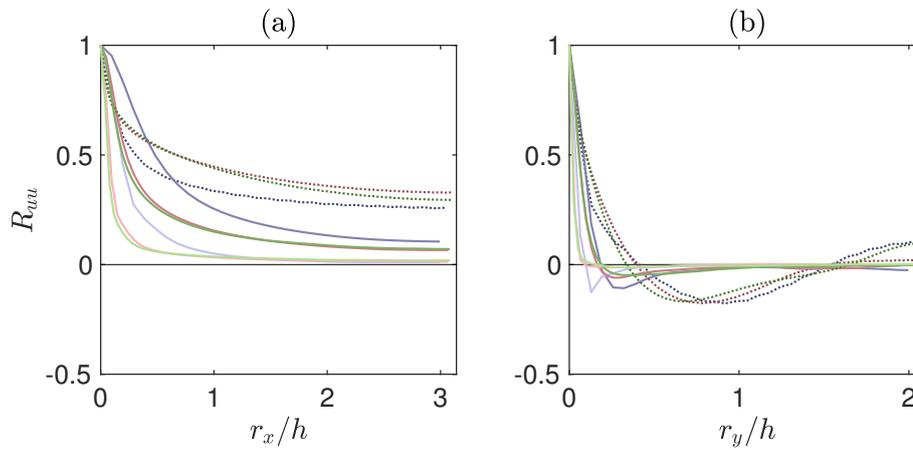
**Figure 5.** Contours of two-dimensional One-dimensional spatial autocorrelation of streamwise velocity at height  $x_2/h \approx 0.1, z/h \approx 0.1$ , from along the simulation R- $2\pi$  streamwise direction (a) and from along the simulation F- $2\pi$  cross-stream direction (b). Dark to light gray lines correspond to contour levels from 0.1 to 0.9 with increments of 0.1. Lines as in Fig. 1.
