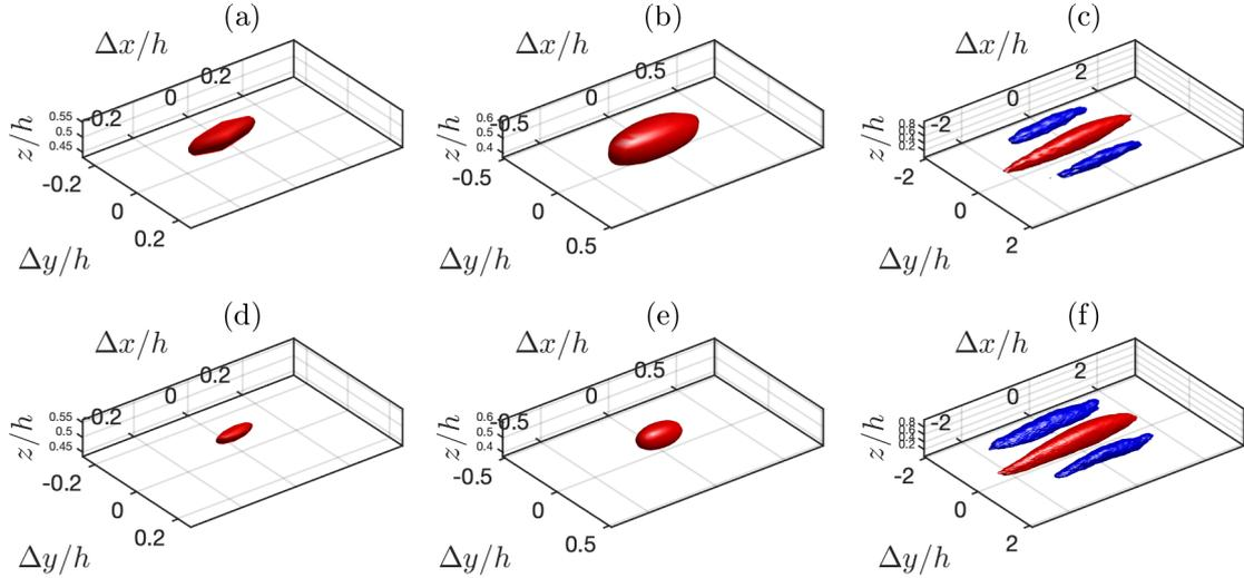
**Figure 10.** Conditionally-averaged flow field from simulations FV64 (a), FV64\* (b), PSFD64 (c), FV160 (d), FV160\* (e) and PSFD160 (f). The conditional event is a positive streamwise velocity fluctuation  $u''/u_*$  at  $\Delta x/h = 0$ ,  $\Delta y/h = 0$ , and  $z/h = 0.5$ . Red iso-surfaces show  $u''/u_* > 0.7$  (top) and  $u''/u_* > 0.65$  (bottom); blue iso-surfaces show  $u''/u_* < -0.55$  (top) and  $u''/u_* < -0.5$  (bottom).
