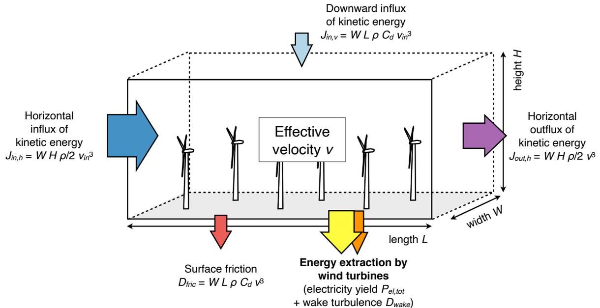
**Figure 1.** Illustration of the Kinetic Energy Budget of the Atmosphere (KEBA) approach to estimate regional wind energy potentials, which considers the fluxes of kinetic energy in and out of a virtual volume that encloses a given region of dimensions  $L \cdot W \cdot H$  to infer limits to electricity generation as well as wind speed reductions. The mathematical formulations of the fluxes are indicated at the arrows.
